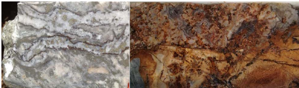
Figure 8-1: Epithermal Deposit Textures in Drill Core Specimens
