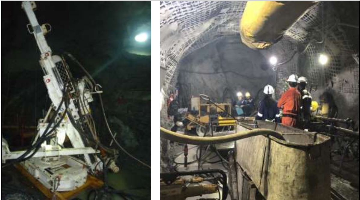
Figure 10-1: Underground Drilling Rig (LM30) in Use at Providencia, and (H200) at El Silencio
