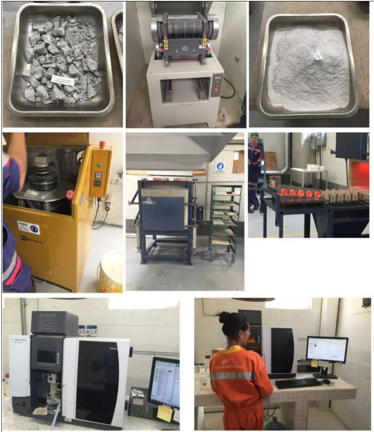
Figure 11-2: Mine Laboratory at Segovia, Showing Crusher, Pulverizer, Furnace and AA Assay Capture
