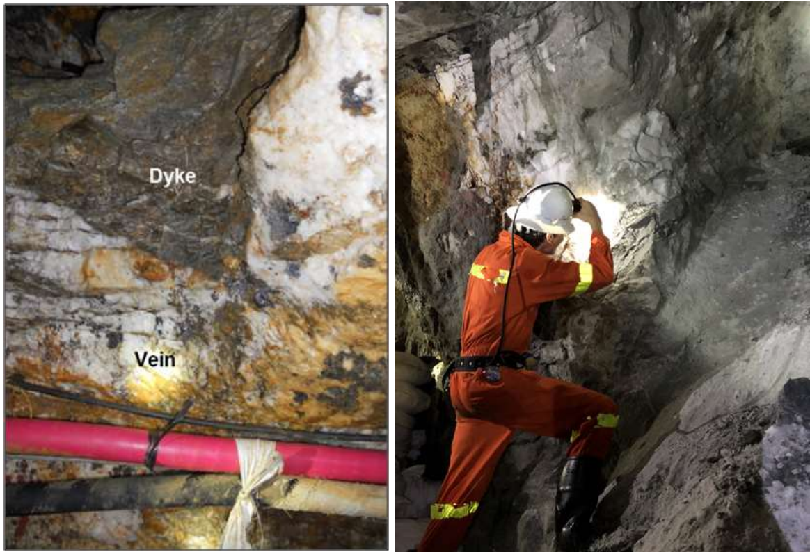
Figure 7-10: Vein Exposures in Underground Workings at El Silencio Showing Relationship with Dikes (left) and Typical Vein Thickness (right)
