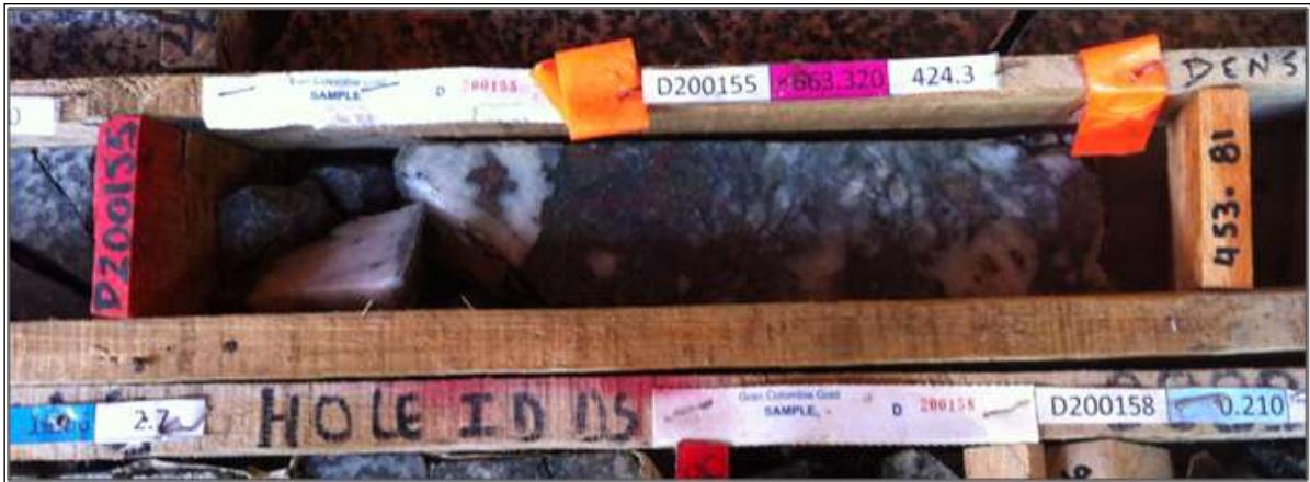
Figure 7-7: Significant Mineralization at Providencia, Intersected in Drillhole DS0089 at 453.54 m, as Observed by SRK
