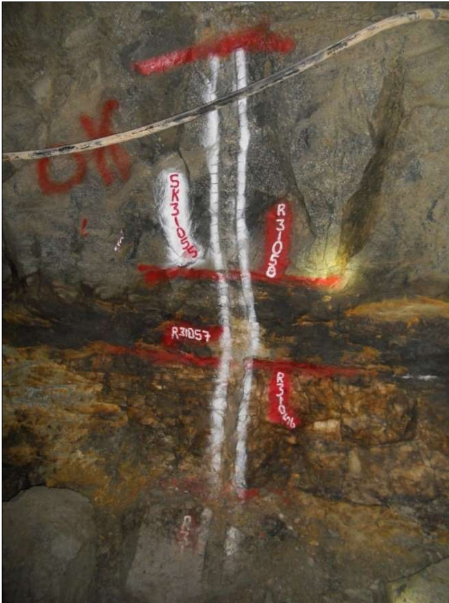
Figure 9-3: Channel Sampling Completed by GCG During 2016 Sampling Program
