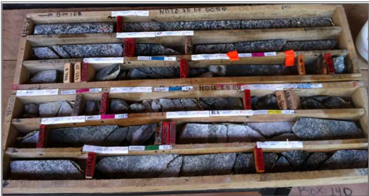
Figure 7-6: Mineralized Zone at Providencia, Intersected in Drillhole DS0089 at 453.20 m, as Observed by SRK (Highest Grade Areas Highlighted by Magenta Tags)
