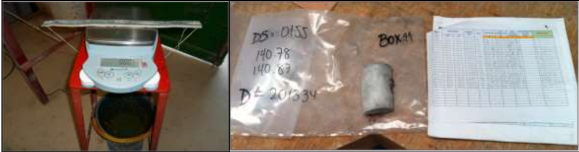
Figure 11-3: Core Sample Coated in Paraffin Wax with Logging Sheet, Prior to Entry to the Database
