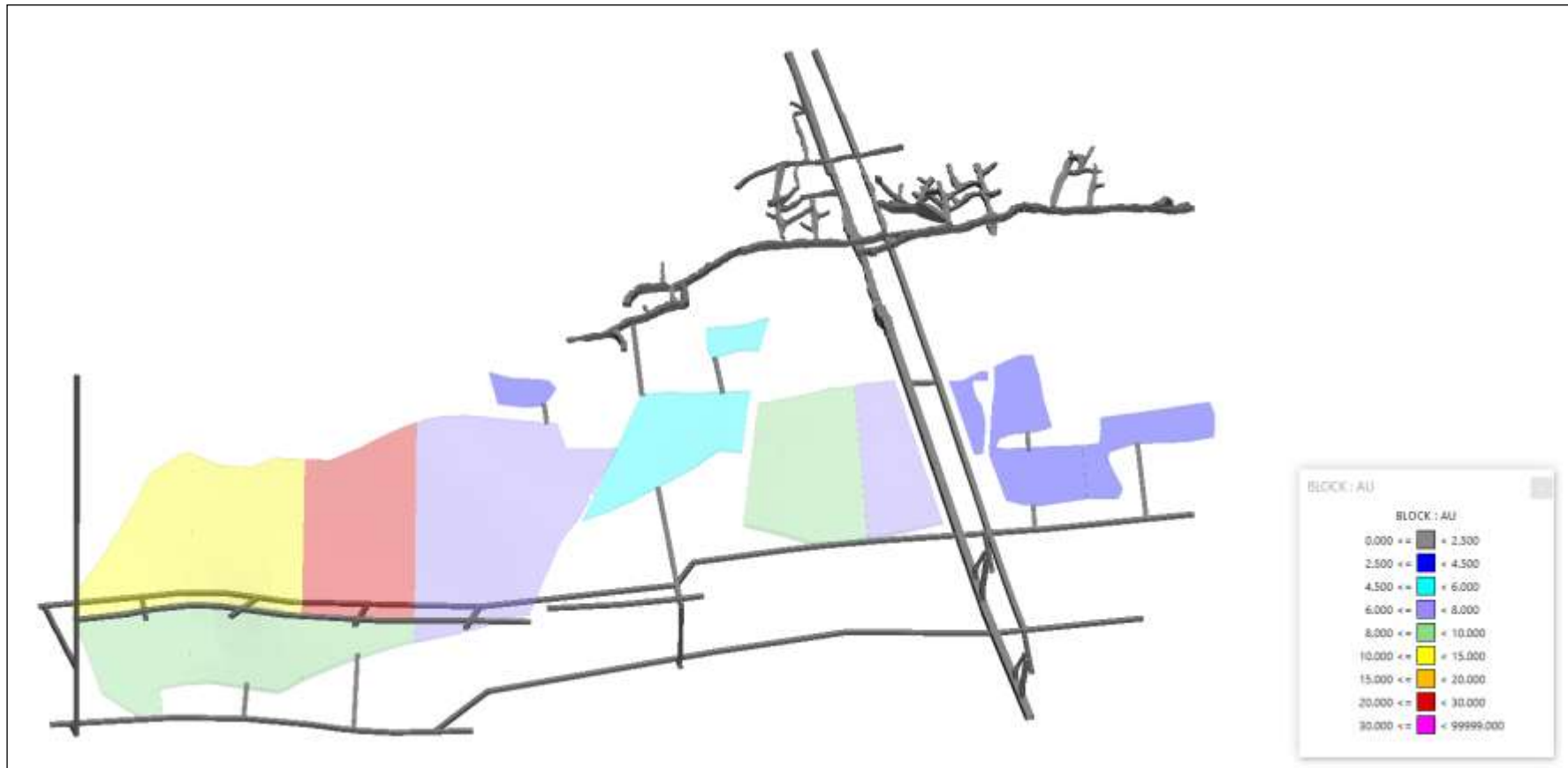
Figure 16-16: Carla Mine Design, Colored by Au Grade (Rotated View)
