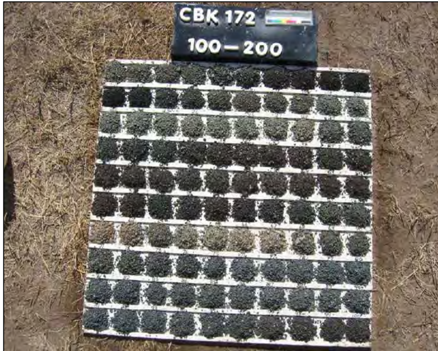
Figure 20. Sieved RC chips collected for metre intervals drilled and available for logging by the geologist.
