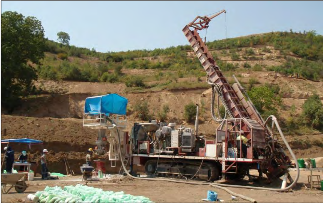
Figure 18. Surface RC Drilling at Shahumyan
