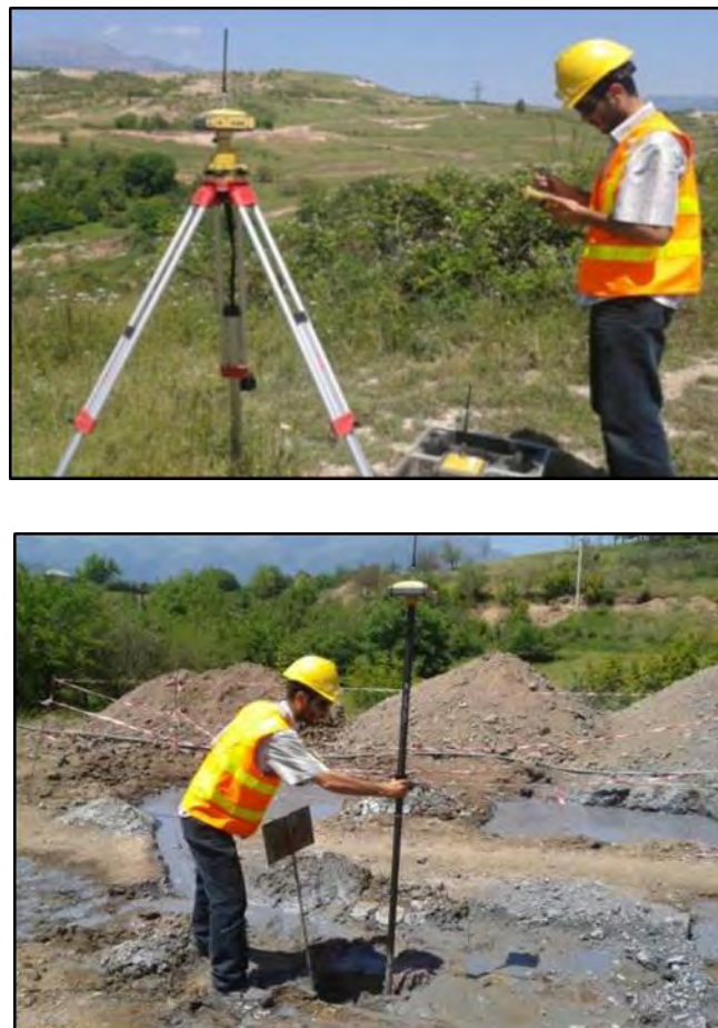
Figure 24. GPS Base Receiver (top) and GPS Rover Receiver (bottom) used for collar surveying
