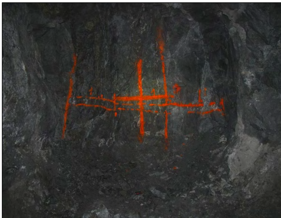
Figure 28. Photo of the face at 703L Vein 3 West, showing sample marks
