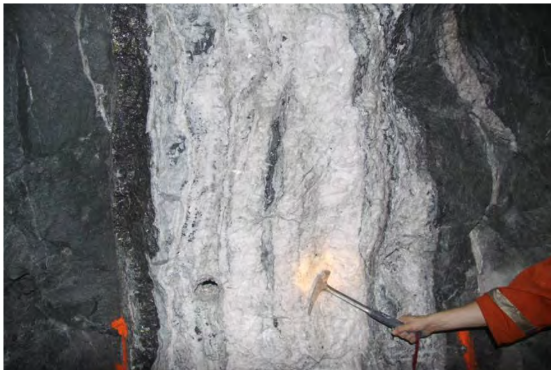
Figure 6. Vein 11 from 775 Level. Massive sphalerite within disseminated chalcopyrite associated with massive calcite infill.
