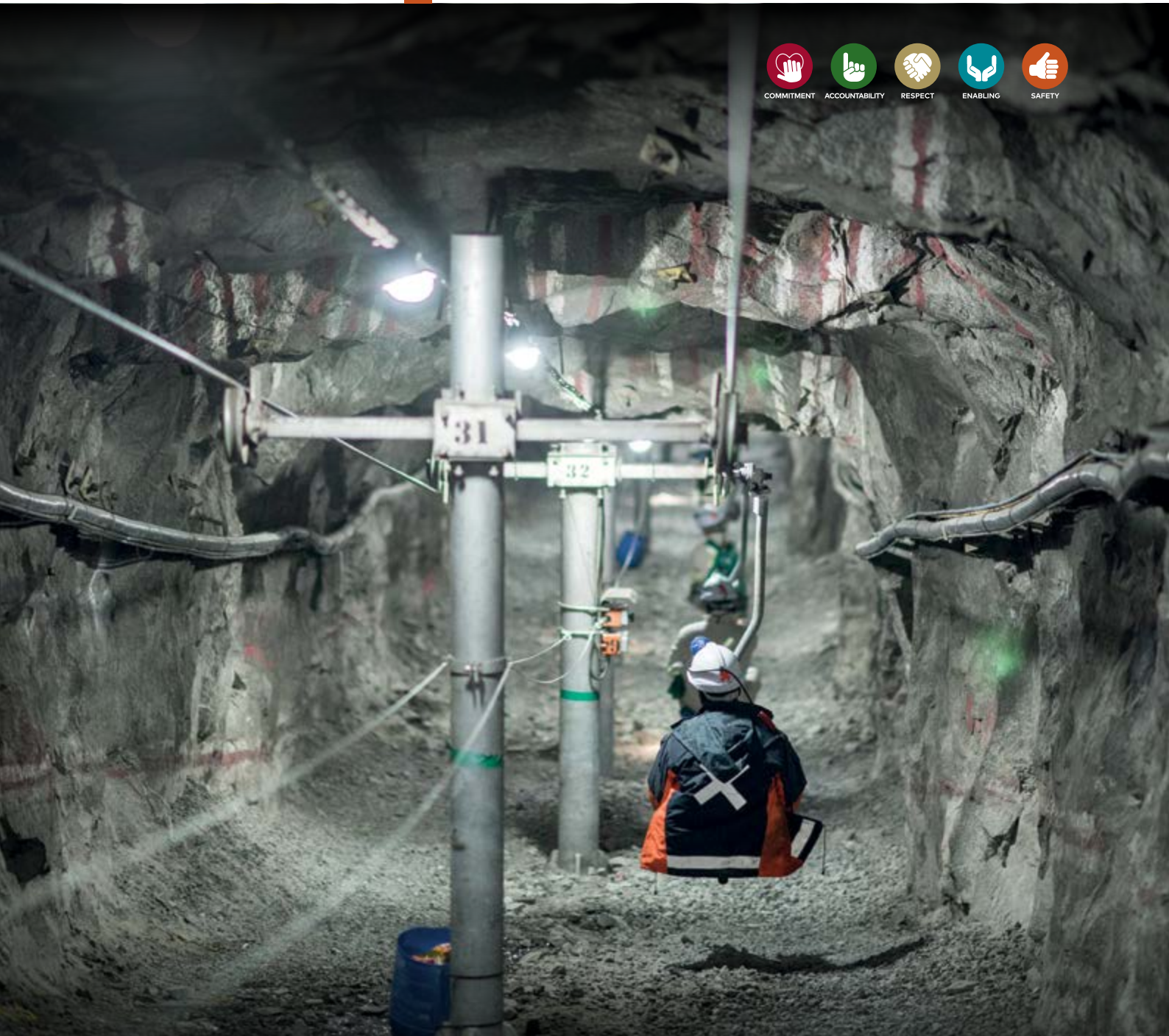
Employees proceeding underground at the K6 SA PGM operation using a chairlift transportation system
