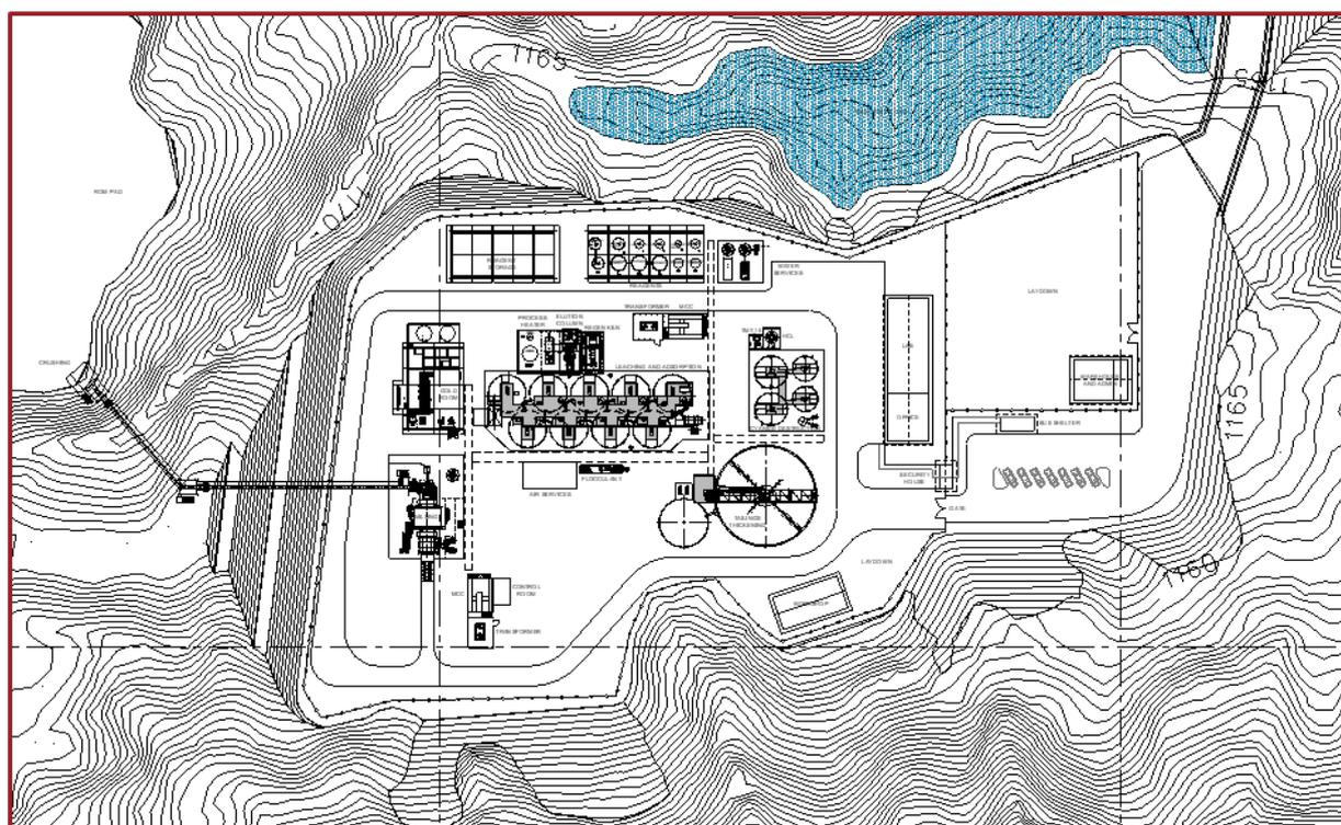
Figure 10 Sihayo Gold Project – processing plant layout
