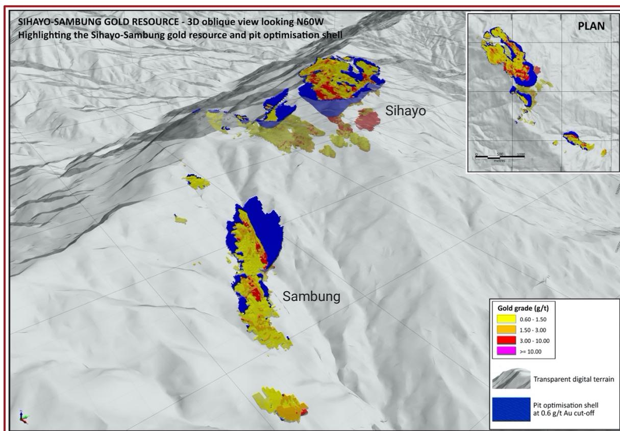
Figure 4 Sihayo Gold Project – 3D oblique view of the Sihayo-Sambung resource and pit optimisation shell
