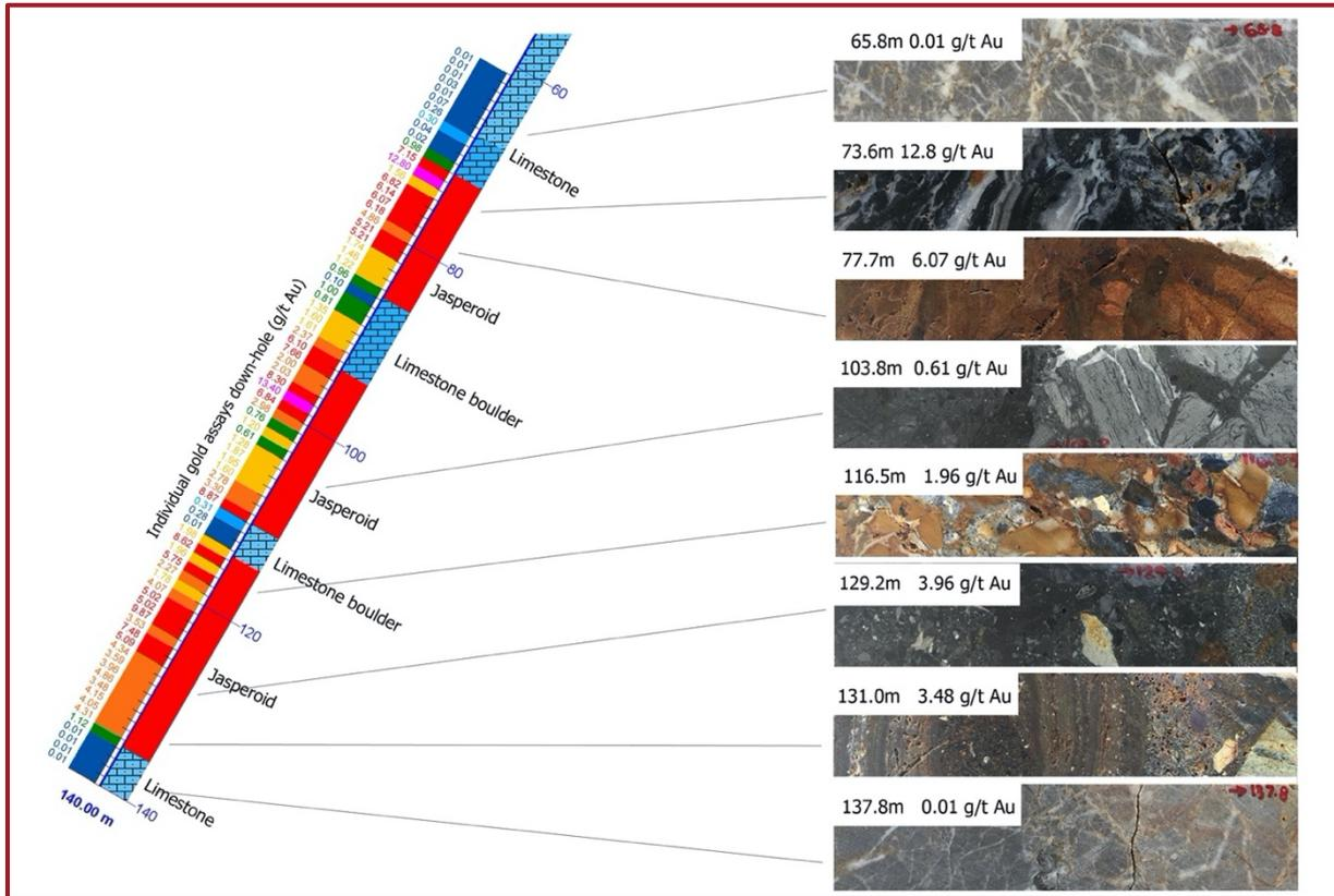
Figure 17 Sihayo Gold Project – SHIDD609 core logging and representative deposit stratigraphy
