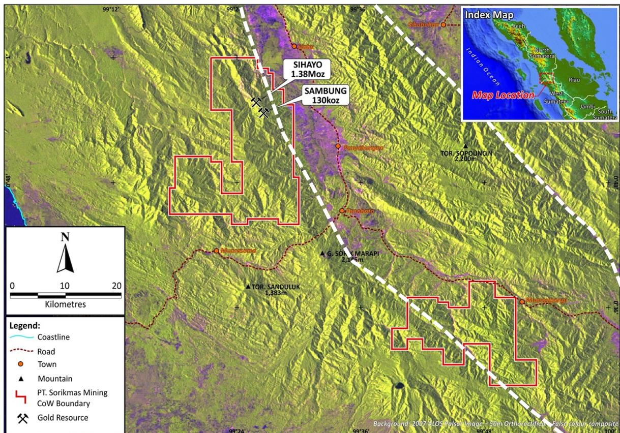
Figure 2 Sihayo Gold Project – CoW boundary map with location of Sihayo and Sambung mineral resources
