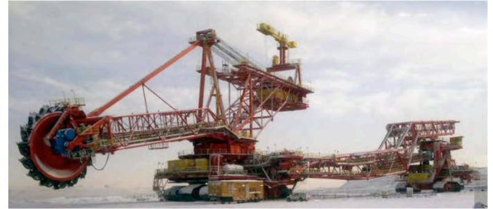
Takraf compact bucketwheel excavator for removing overburden with lowest unit cost
