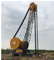
RTEC trench cutter bulk sampling rig
