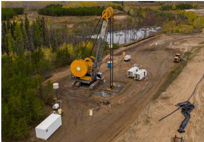
RTEC trench cutter bulk sampling rig
