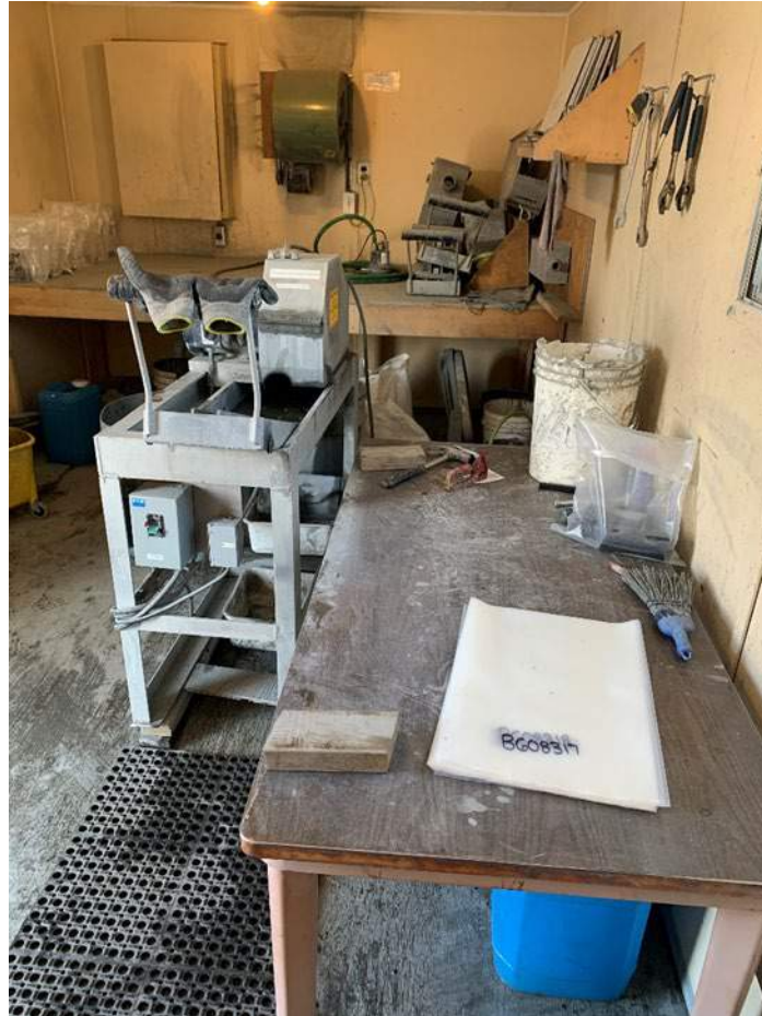
Figure 11-1: Purpose-designed Vancon diamond-bladed core saw with pre-marked sample bags
