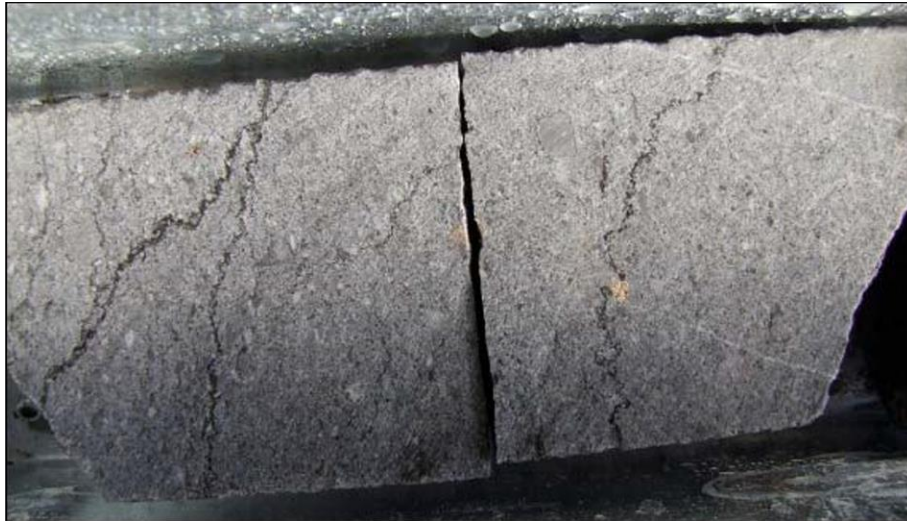
Figure 7.5 – Typical S1 Unit: Fine-Grained Calcirudite with Stylolites
