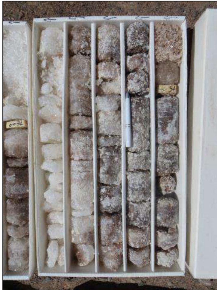
Photo 7-12: Porous Halite shown in core from borehole PP1-D-22, at 78 m depth.
