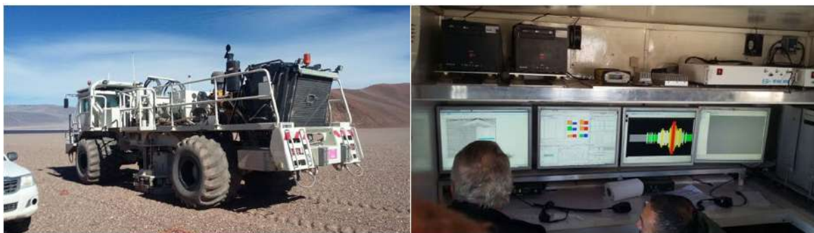
Photo 9-2: Vibroseis Sercell with seismometers set up at 20 m spacing (left). Interior controls for the seismic equipment (right).
