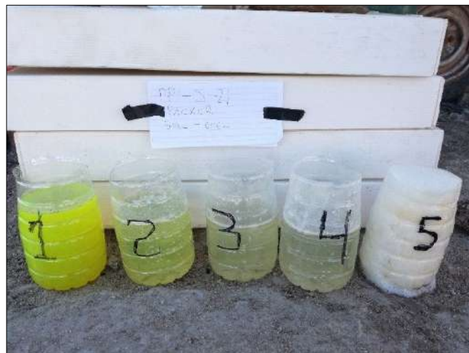
Photo 11-7: Progressive clearing of the tracer from the packed interval, as purging proceeds.
