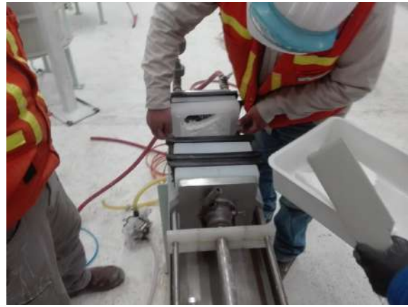
Photo 13-7: Pilot settler test and pilot press filter filtration tests.
