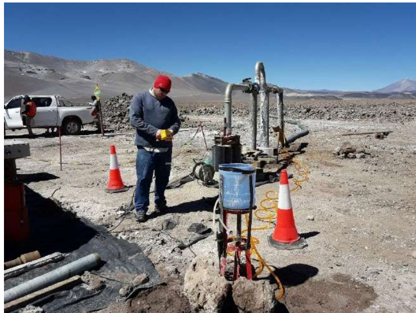
Photo 11-8: Pumping test setup at well PB2-R-3.
