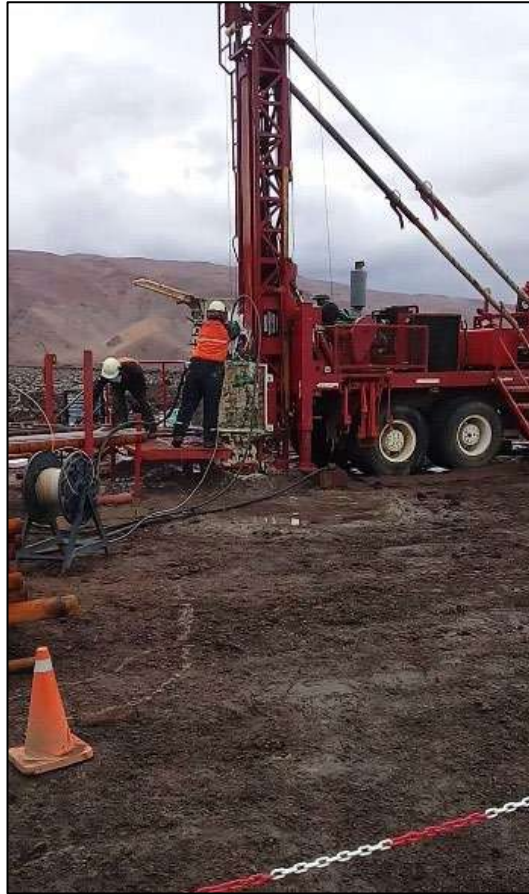
Photo 11-6: Packer assembly being placed in PP1-D-17.
