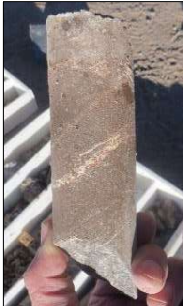
Photo 7-9: Core from the hydrogeological basement, with a dip varying from 5 to 40 degrees.
