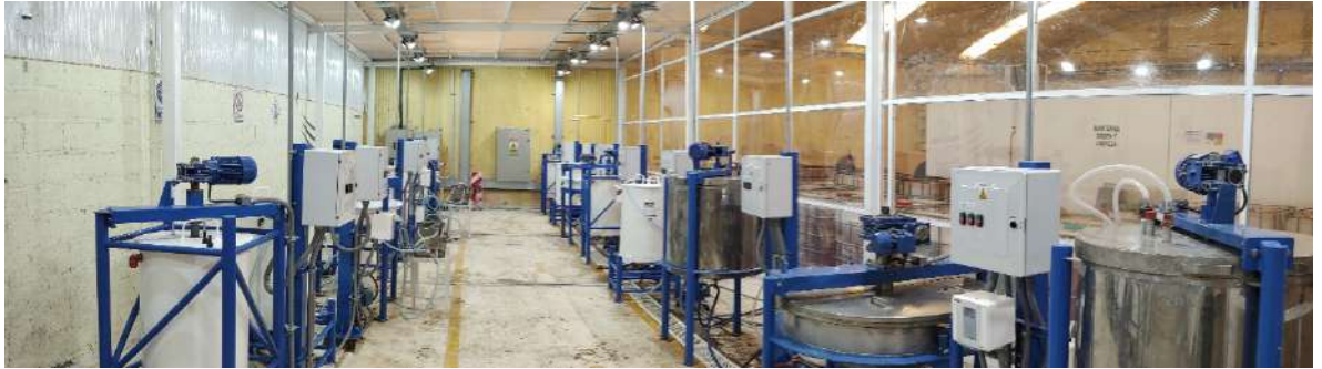
Photo 13-6: Facilities for testing the difference stages of \text{Li}_2\text{CO}_3 production in the \text{Li}_2\text{CO}_3 Pilot Plant.
