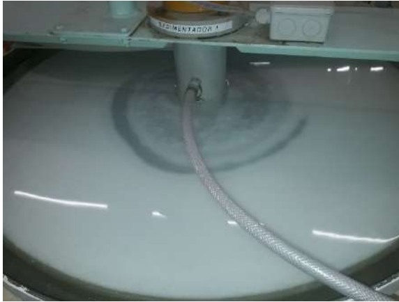
Photo 13-7: Pilot settler test and pilot press filter filtration tests.
