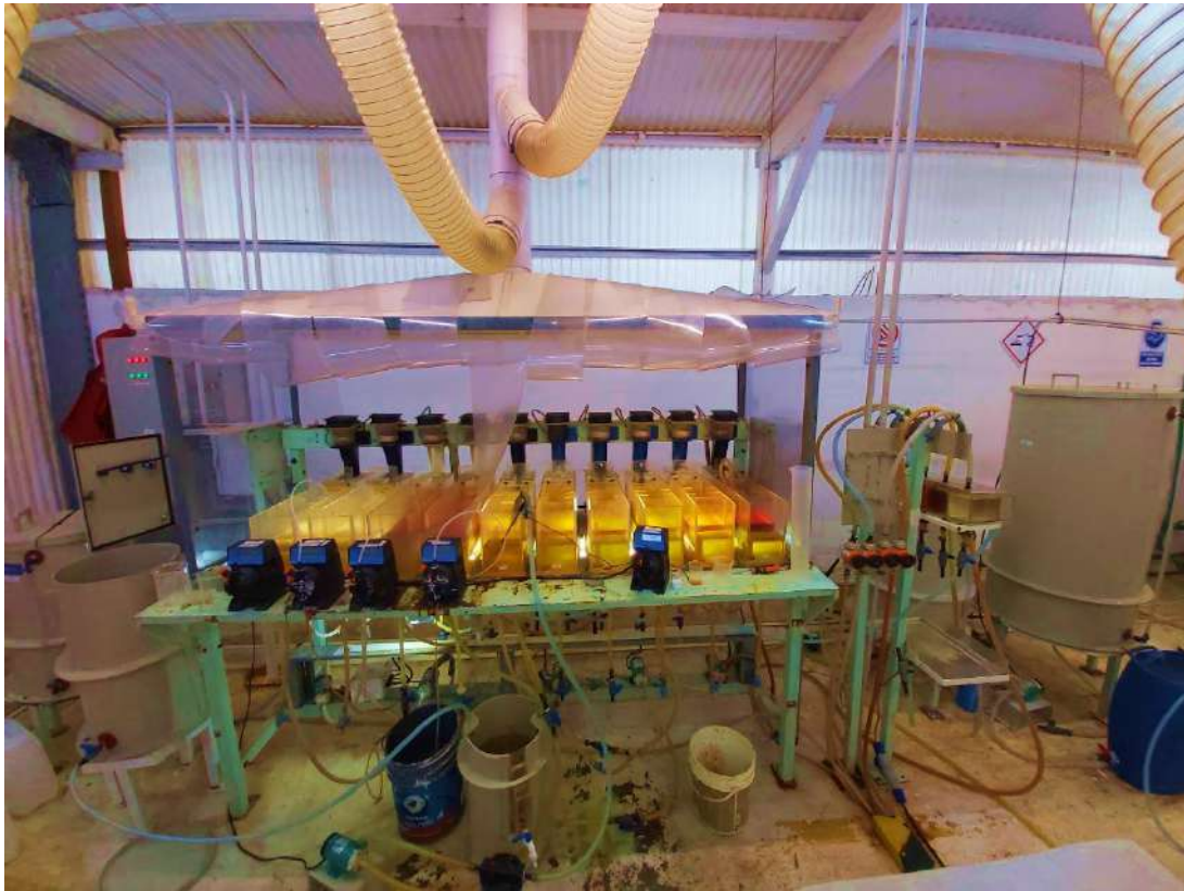
Photo 13-5: SX-scrubbing and stripping tests.
