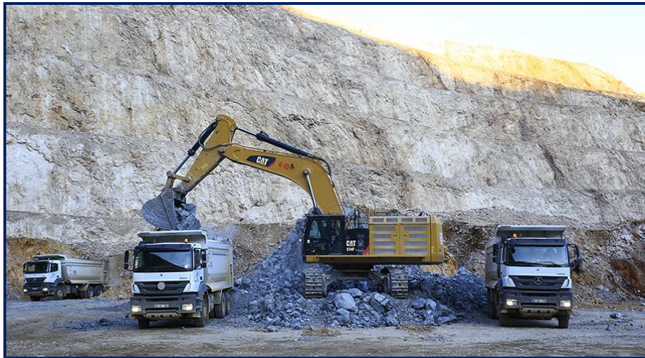
FIGURE 16-16 CAT 374 EXCAVATOR LOADING MERCEDES ACTROS 3340 TRUCKS
