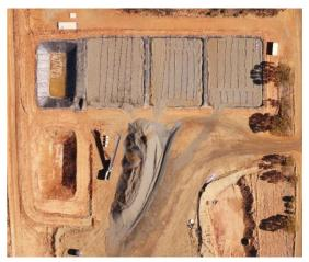
Plan view of the three heap leach pads, prestacked scats, with the aeration piping and PLS collection pond (LHS)
