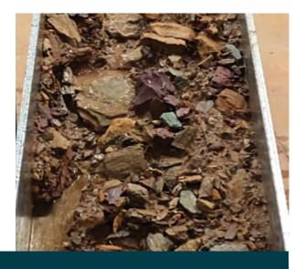
Erosion and rehabilitation experts tested mixtures of rock and soil to find the best combination for capping and revegetating landforms.
