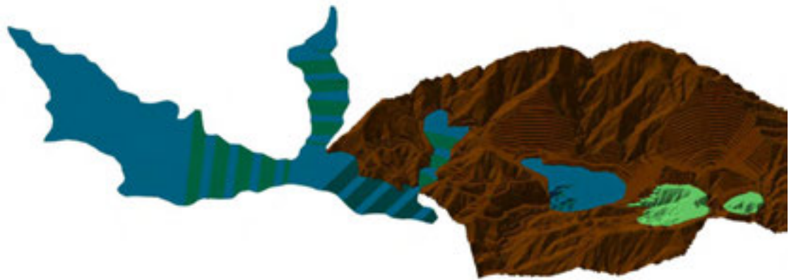
Figure 16-25: End of the Fourteenth Year of Production (Year 16 – 2035) - Backfilling into Gremi
