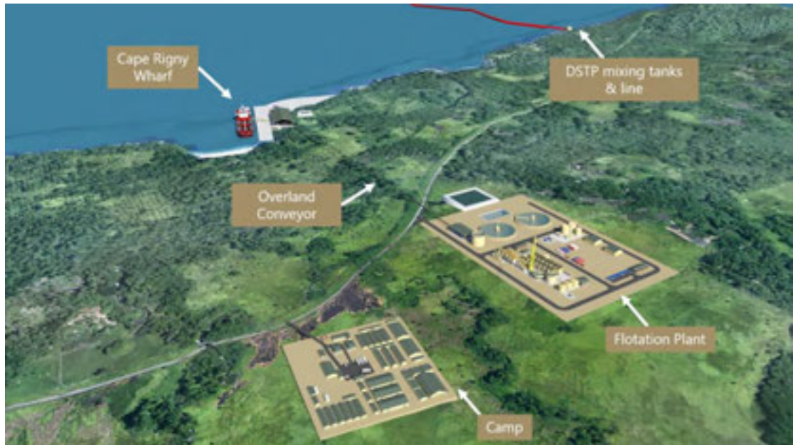
Figure 1-7: Coastal Facilities Conceptual Layout
