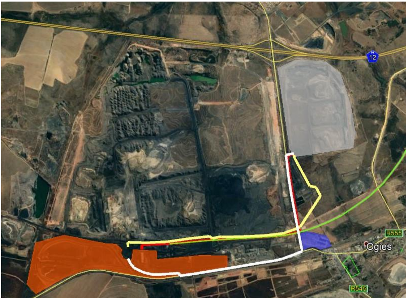
Figure 8: Map indicating conceptual alignment of proposed discard transport alternatives. A public road route in white, a proposed mine road crossing the South32 property in yellow and proposed new conveyor route in red. The alignment of an existing coal conveyor is indicated in green.
