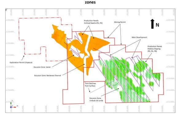
Figure 1: Plan view of Muga-Vipasca mining panels including access development and exclusion
