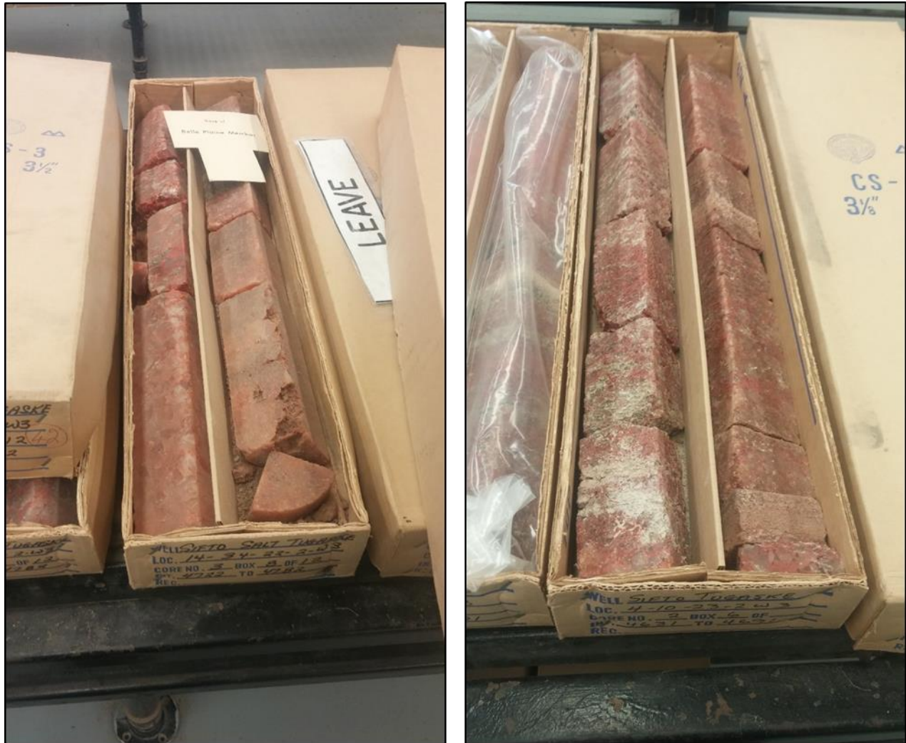
Figure 8: Preserved Potash Core From The 1960's Exploration Programs In The Tugaske Area
