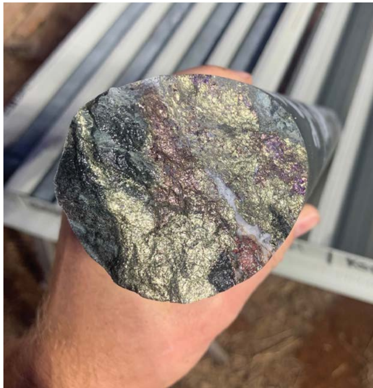
Cross section of mineralised core from diamond hole KSDD007 drilled at Boda, showing 2cm-thick bornite-chalcopryite-quartz vein at 385m downhole.
