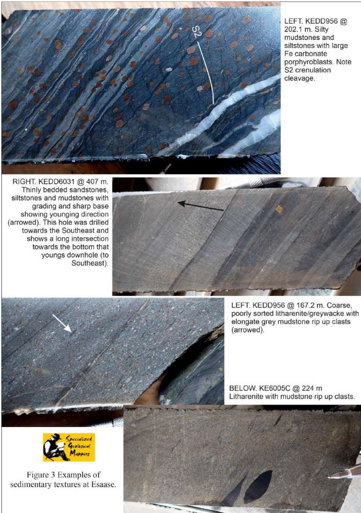
Figure 7-8 Examples of Sedimentary Textures at Esaase Source: Pratt, 2021
