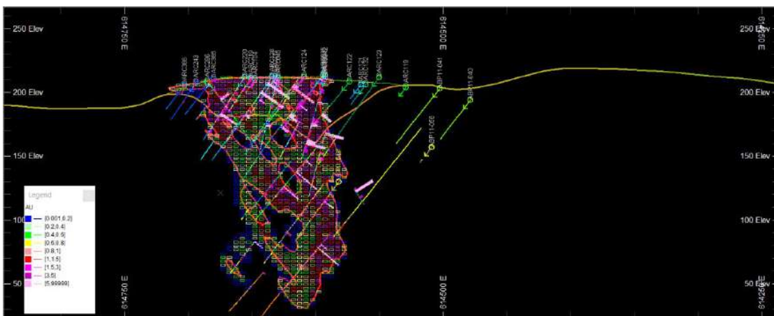
Figure 14-34 Above Au Grade Estimates, Cross Section 714170N Note: Colour-coded according to legend shown. Grade envelope outline shown in red.
