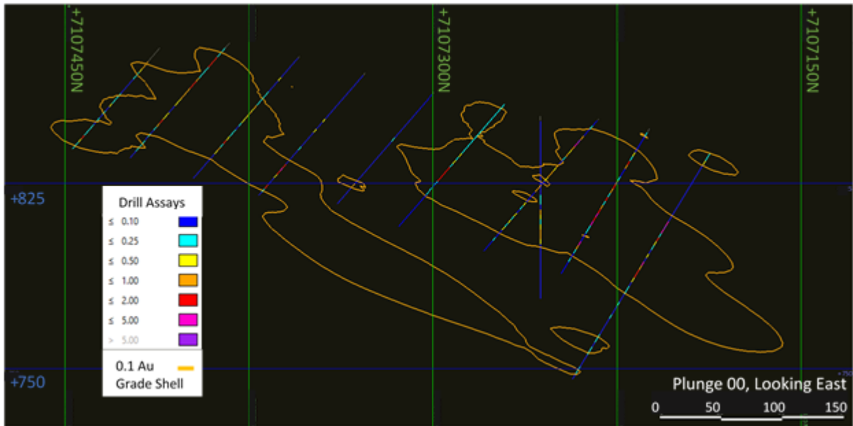
Figure 14-5 Example Section A-A' of Lucky Looking East Showing Grade Shell (Orange) Constrained to Higher Au Mineralization in Assay Drill Data
