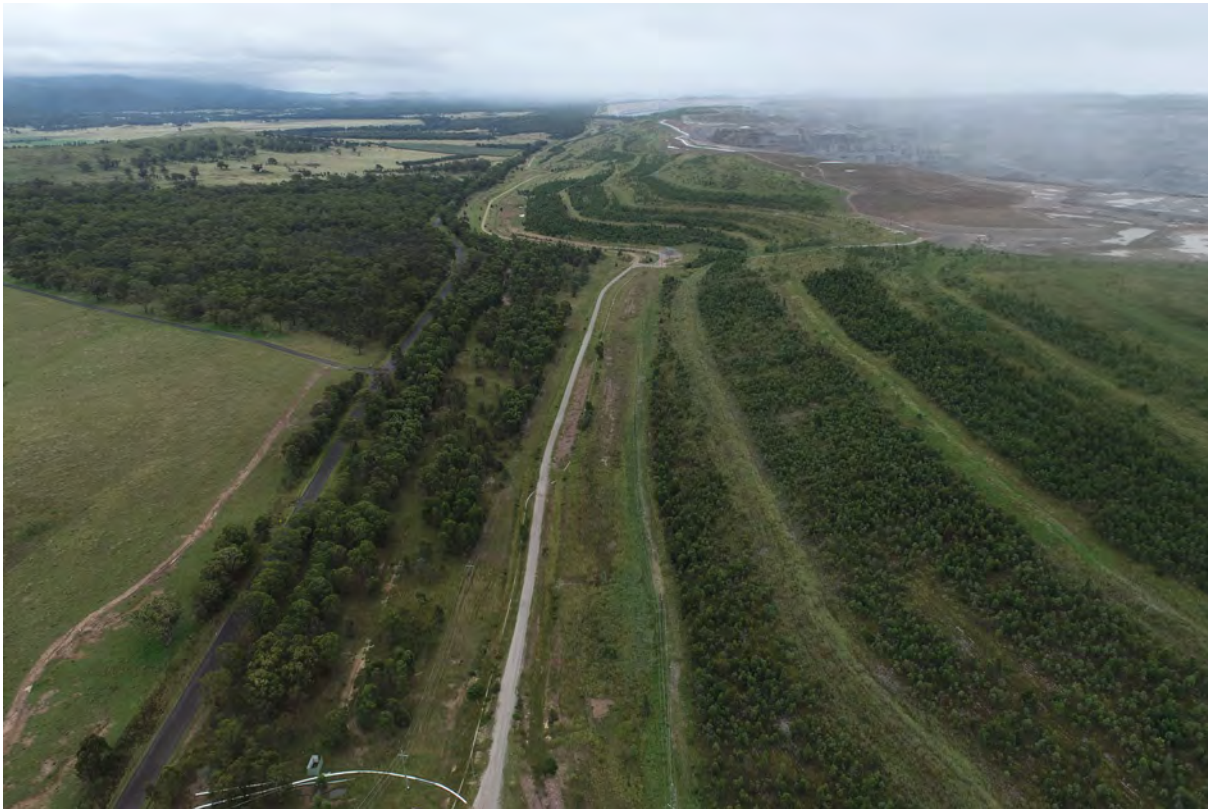
Photo 10 Vegetation establishment on the Noise and Visual Bund (foreground), and completed 2021 rehabilitation (background).
