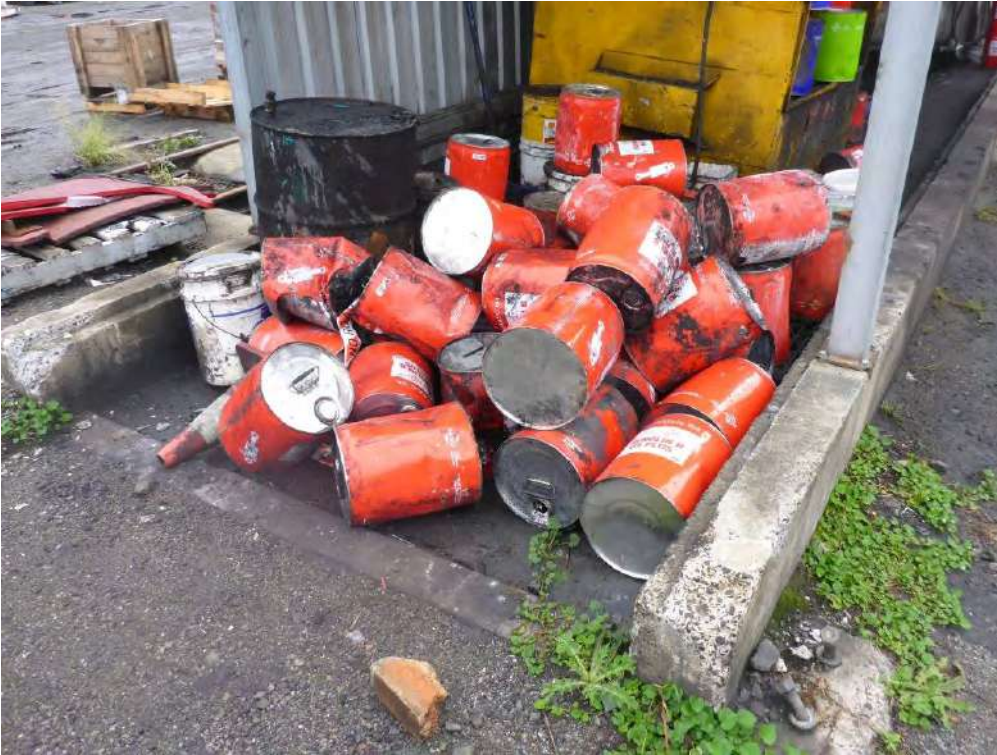
Photo 3 Hydraulic oil container stored on the side within bunded area. Improvement Required.
