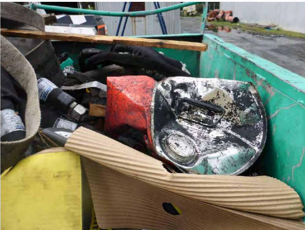
Photo 4 Hydraulic oil container should not be stored in general waste
