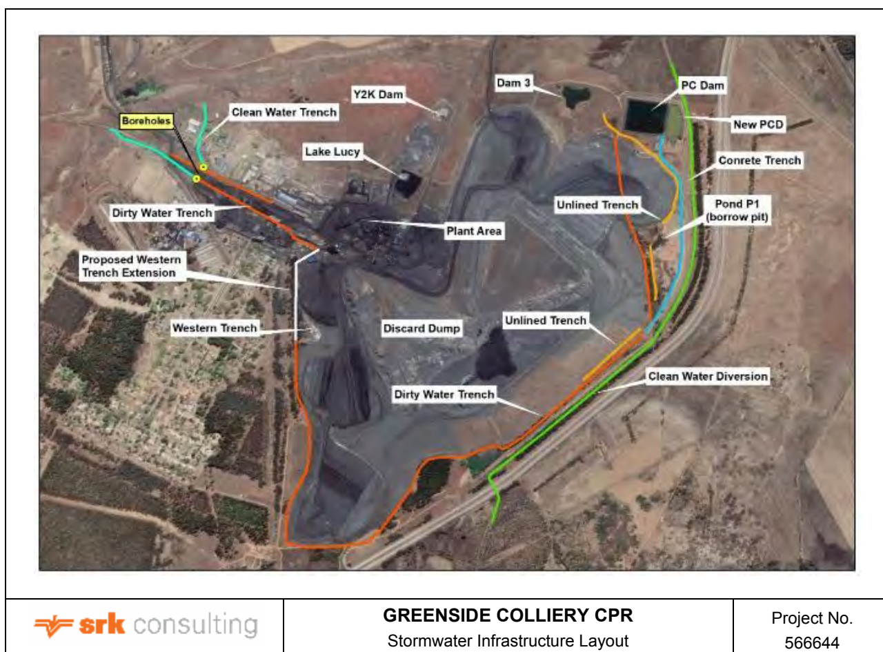
Figure 16-1: Stormwater Infrastructure Layout at Greenside Colliery
