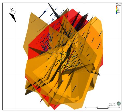
Figure 13-1: Oblique 3D view showing main faults (2 and 14 in red) and other modelled faults (orange) and drillholes coloured by Ni(S) domain
