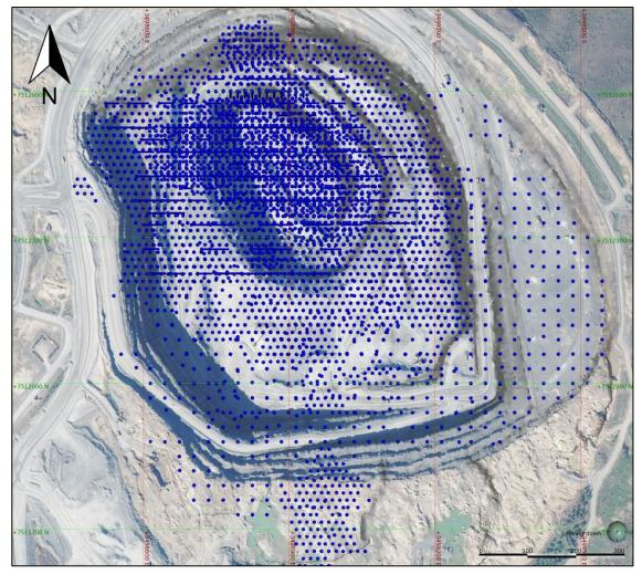
Figure 9-2: RC drillhole collars and topographic surface with satellite imagery as of end-2019
