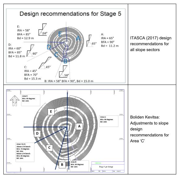
Figure 14-12: Slope design parameters by design sector
