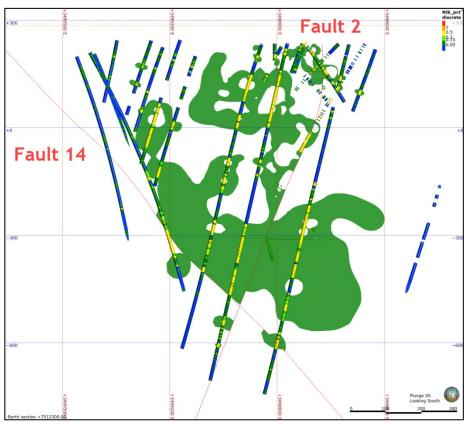
Figure 13-3: Cross-section (Y: 7512300) showing main faults (2 and 14) with low-grade Ni domain and drillholes coloured by Ni(S) domain
