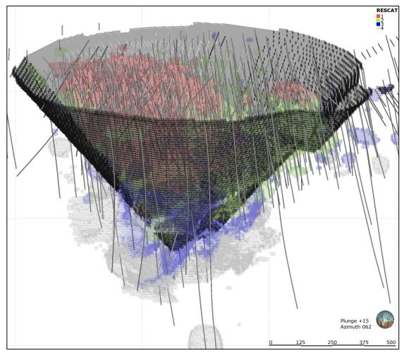
Figure 13-21: Whittle pit shell used for Mineral Resource reporting and block model coloured by Mineral Resource Classification
