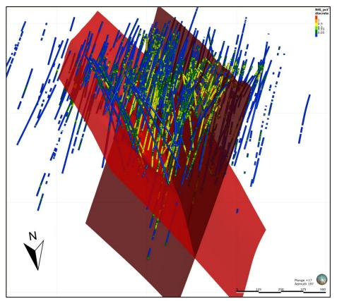
Figure 13-2: Oblique 3D view showing main faults (2 and 14 in red) and drillholes coloured by Ni(S) domain
