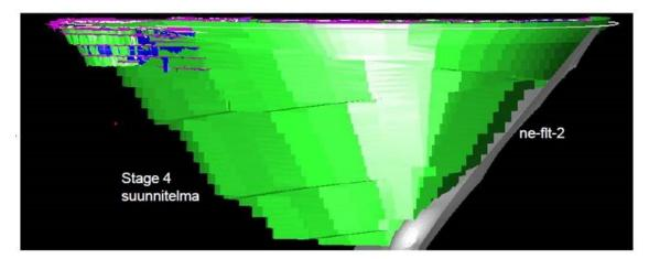
Figure 14-13: Stage 4 pit design with NE-FLT-2 Structure located near east wall
