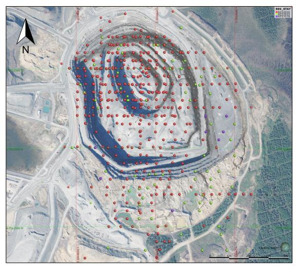
Figure 9-1: Diamond core drillholes completed at Kevitsa prior to MRE 2018 coloured MRE database (red = used for 2011, 2016, 2018 MRE; green = used for 2016, 2018 MRE only; purple = used for 2018 MRE only) and topographic surface with satellite imagery as of end-2019
