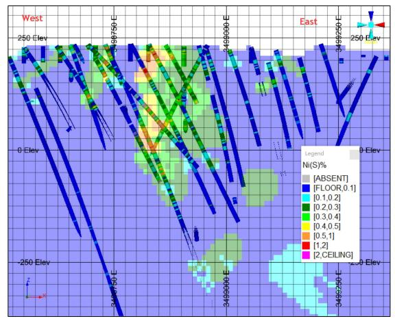
Figure 13-16: West-east cross section (Y: 7512500) of Ni(S) estimate block model and sample composites (section thickness 20 m)
