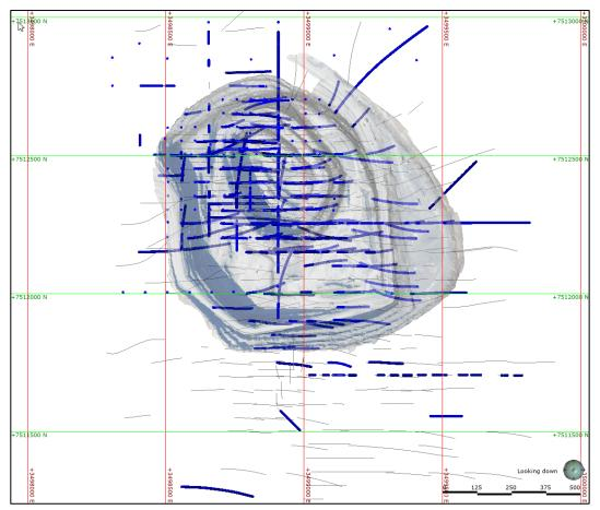
Figure 10-2: Plan view of Kevitsa pit showing holes containing density data (blue) (Source: SRK, 2019)
