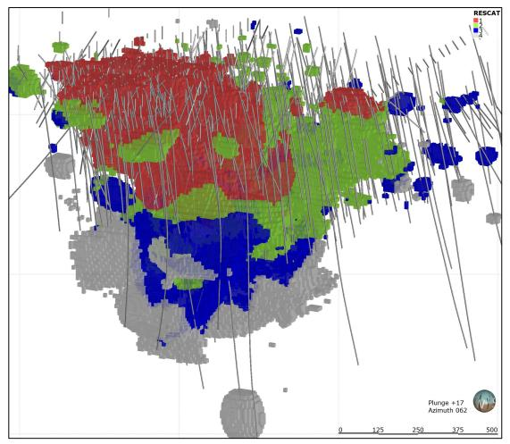
Figure 13-17: 3D view of the block model (mineralisation blocks only) coloured by Mineral Resource classification category (1 = Measured, 2 = Indicated, 3 = Inferred, 4 = Unclassified)
