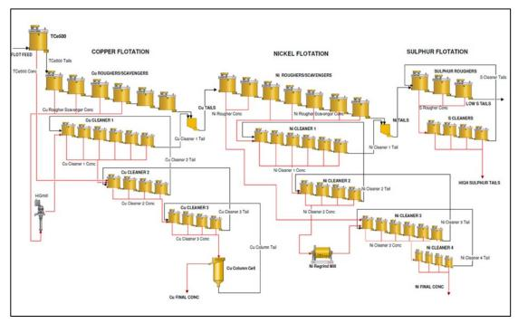
Figure 15-2: Kevitsa Cu and Ni Flotation Circuits (Source: Boliden, 2019)
