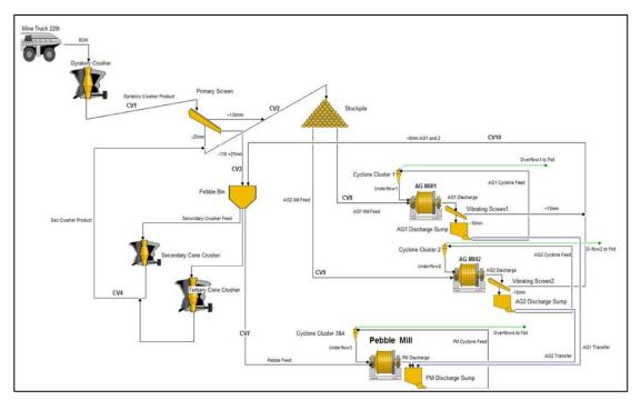
Figure 15-1: Kevitsa Crushing and Grinding Circuits (Source: Boliden, 2019)
