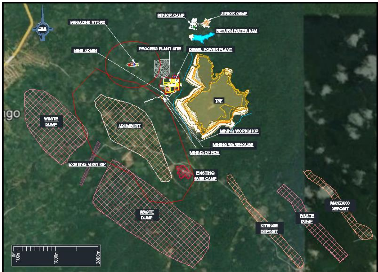
Figure IV: Adumbi Key Infrastructure and Site layout
