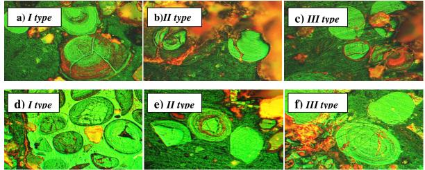
Figure 5. Structure of fractions:a, b, c – 3÷1,25 and d, e, f - 5÷3 mm l, ll and lll types of Lisakovskiy ores. Reflected light, zoom 10x
