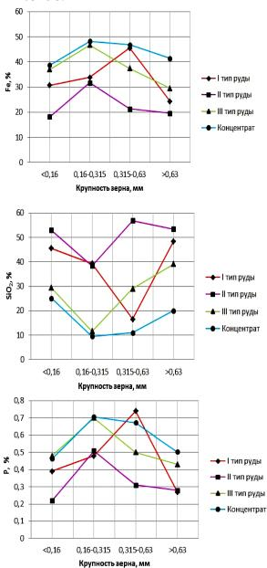
**Figure 1**. Quality of I, II and III types of Lisakovskiy ore and concentrate
