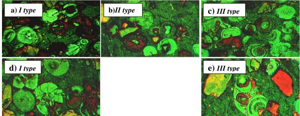
**Figure 4.** Structure of fractions: a, b, c – 0,63÷0,4 mm I, II and III types of Lisakovskiy ores; d, e – 1,25÷0,63 mm I and III types of Lisakovskiy ores. Reflected light; a, c - zoom 10x, b, d, e - zoom 5x
