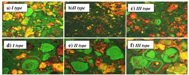
Figure 3. Structure of fractions: a, b, c - 0÷0,2 mm and d, e, f - 0,4÷0,2 mm I, II and III types of Lisakovskiy ores. Reflected light; zoom 10x
