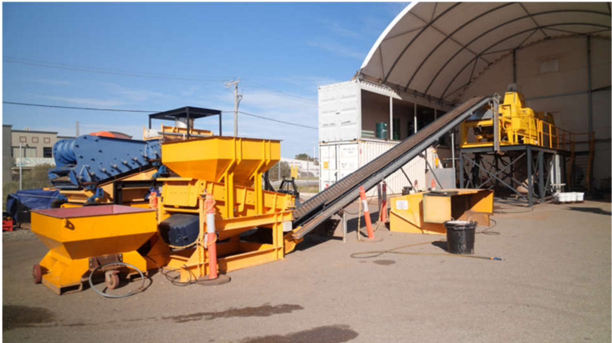
Figure 2: Ore sorting facility used during testwork is the same size proposed for use at Kayelekera
