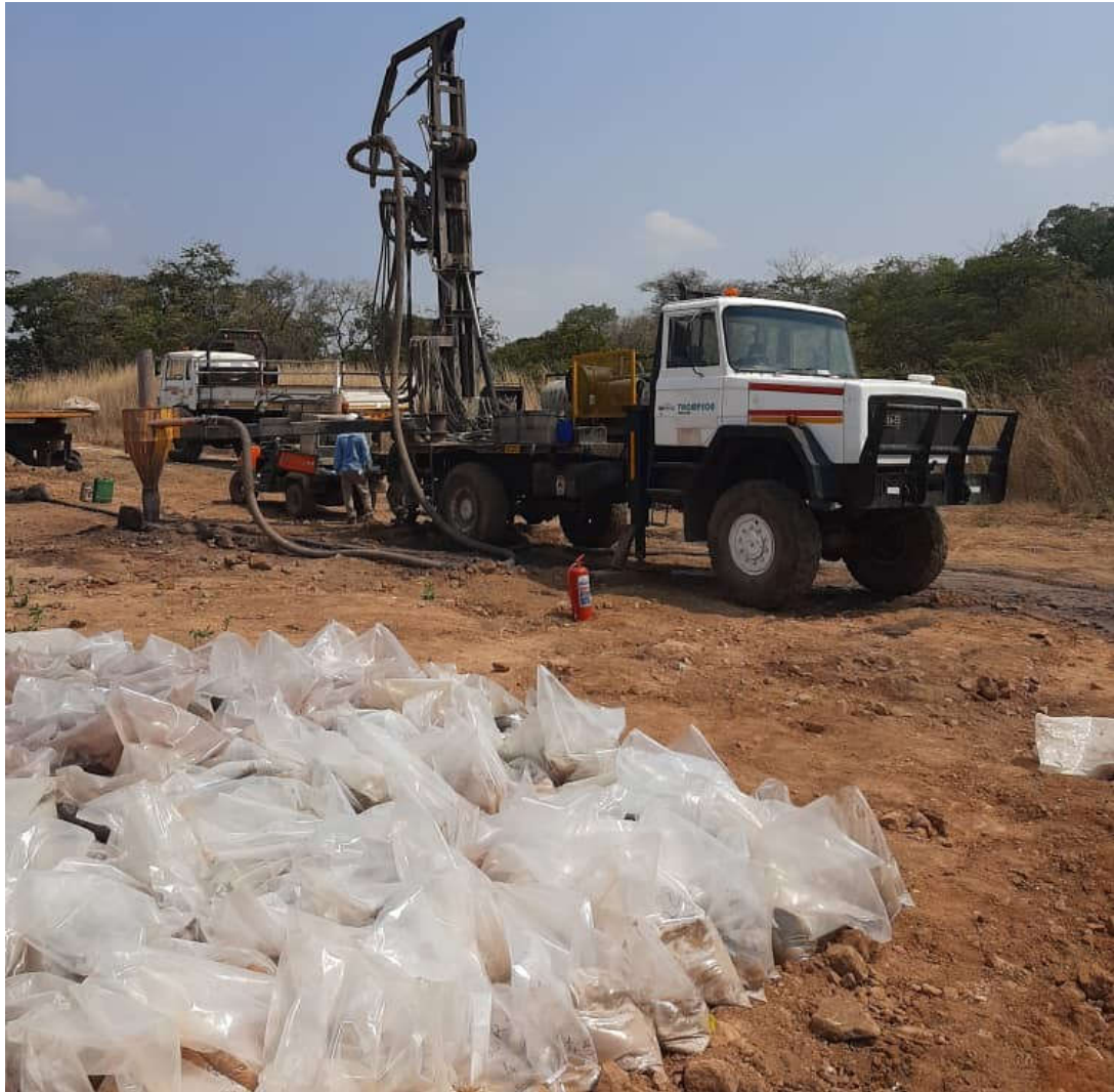
Figure 4: RC Drilling on the south-east corner of the pit
