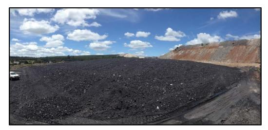
Figure 6: Carey's low ash "Enviro" coal stockpile, track rolled in several lifts and batters reduced to limit ingress of air in line with SOP 4868-SE-SOP1027 ("Spon Com") guidelines
