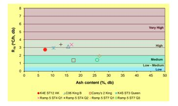
Figure 4: R<sub>70</sub> self-heating relationship with ash content for coal samples from Meandu Mine, showing intrinsic spontaneous combustion propensity classes based on Queensland conditions
