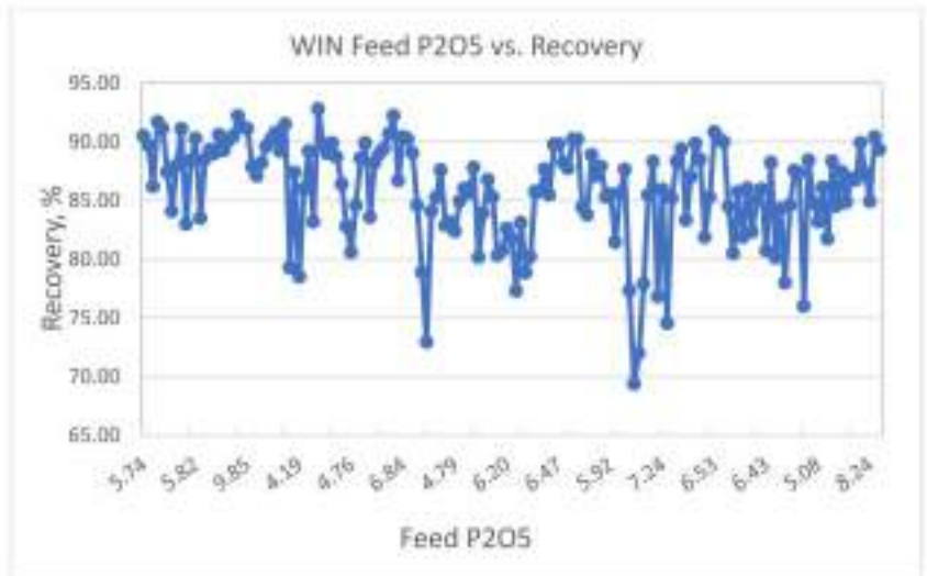
Figure 10-3: Wingate Feed P 2 O 5 Grade vs. Recovery%
