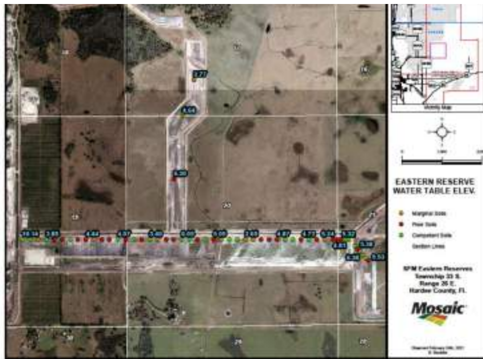
Figure 13-7: Dragline Walk Path Soil Penetration Testing and Piezometers
