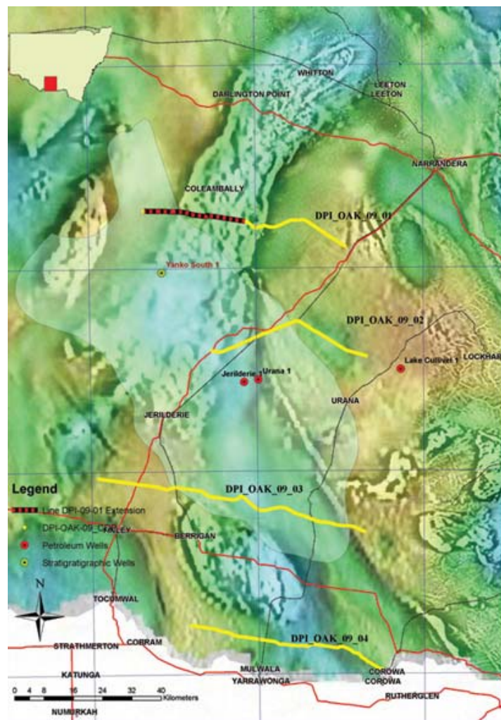
Figure 12.3. Location of 2009 Oaklands Basin seismic profiles. Transparent shape delineates the recognized outline of the basin (from: http://www.resources.nsw.gov.au/geological/about/geophysical-surveys/oaklands-basin-2d-2009-seismic-survey ).
