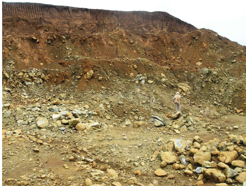
Figure 3.2 Typical nickel laterite profile at HM showing the red limonite (top), mottled saprolite (middle) and ultramafic bedrock (bottom).
