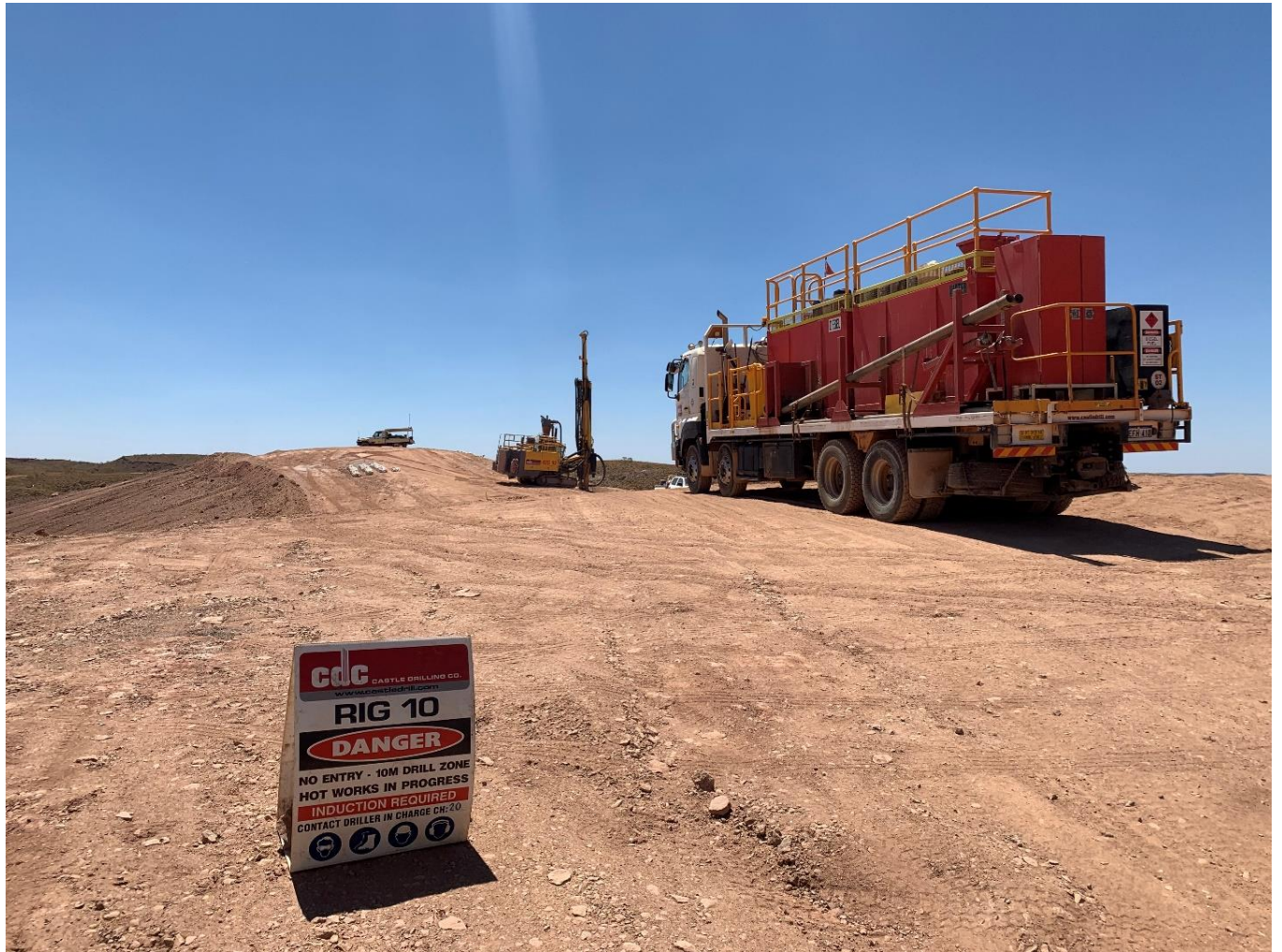
(Figure 1: Grade control drilling continues at the Edwards Lease.)
