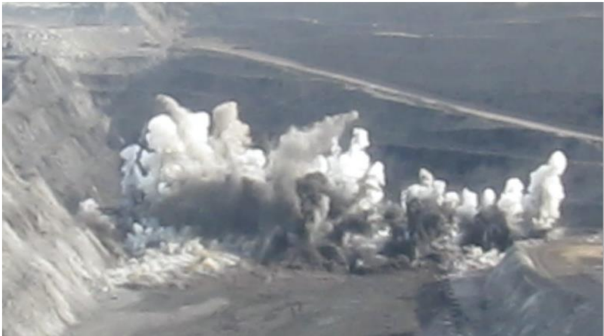
Figure 16-6: Sunrise Main Pit (blasting in northeast working face, looking east)
