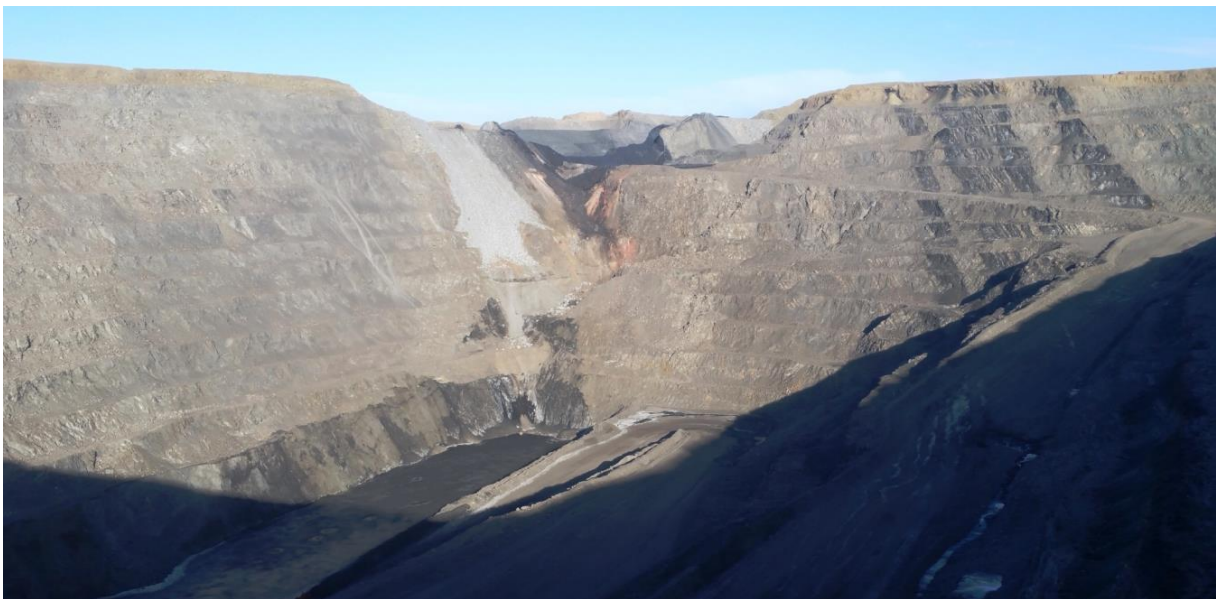
Figure 8-1: The coal seams and stratigraphy are generally very continuous at the Sunset Pit. Extensive tight folds, steeply inclined and overturned beds and large displacement faults are not observed at the Sunset Pit.
