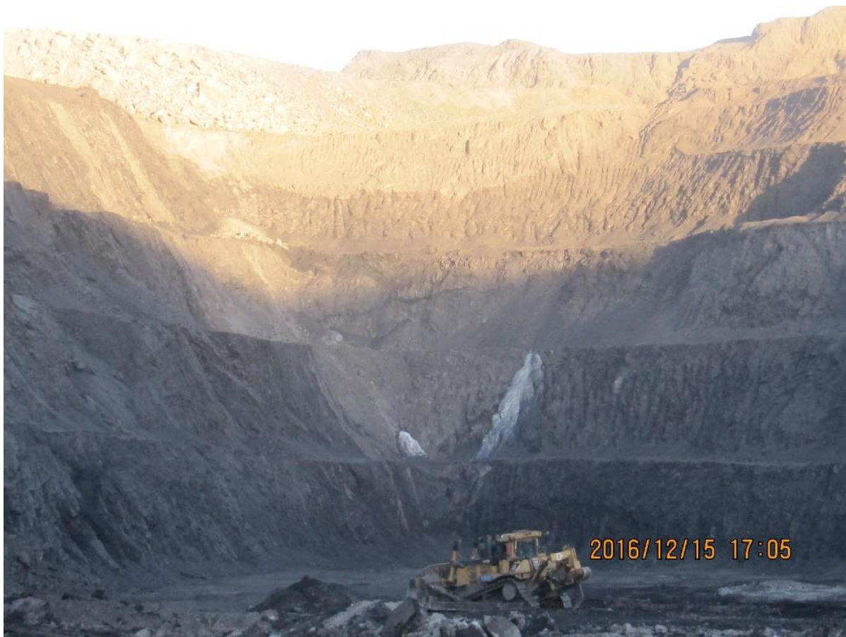
Figure 16-15: Frozen Seepage Through Pit Wall of the Sunrise Pit
