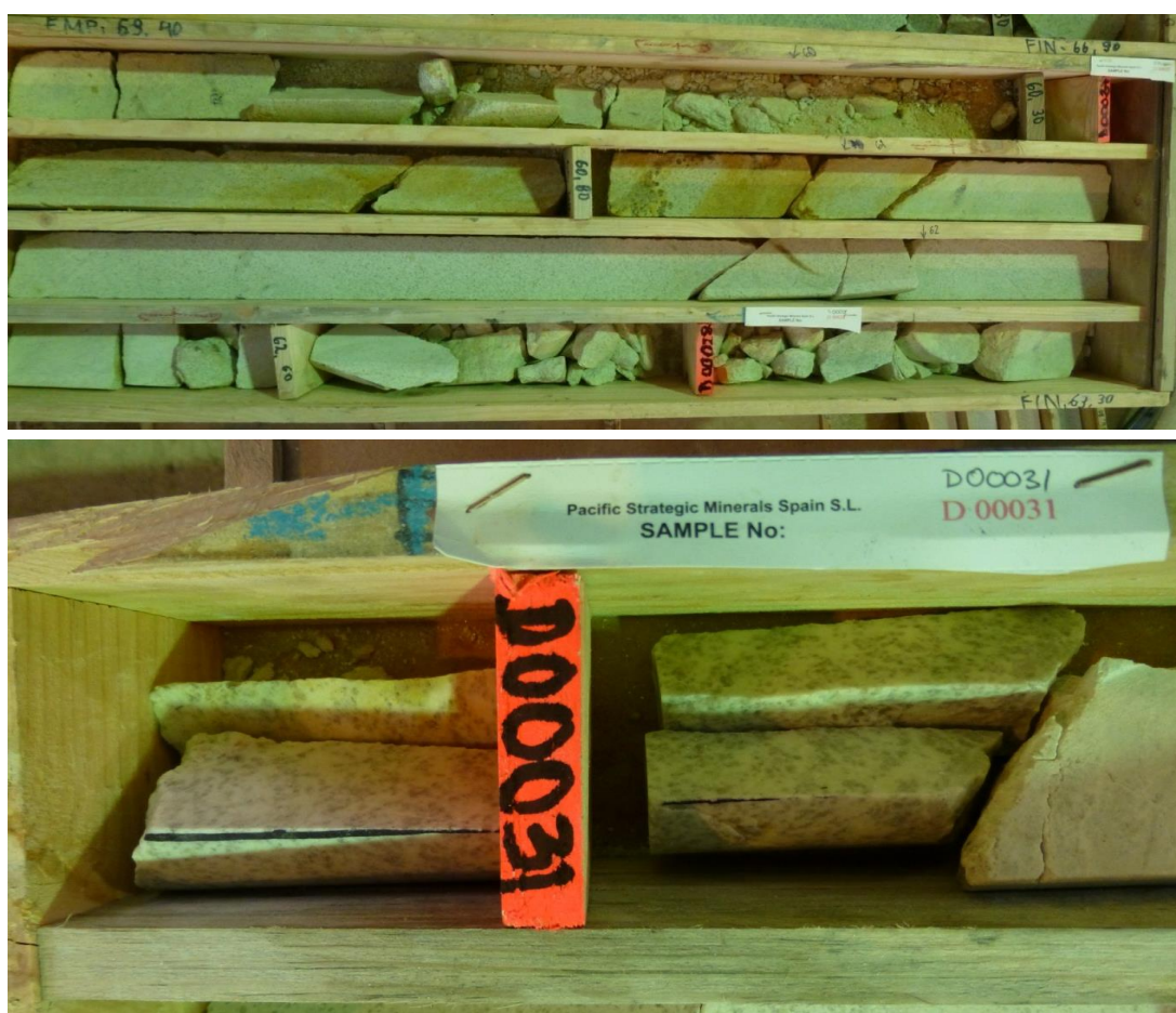
Figure 11-2: Core sampling procedures at Penouta
