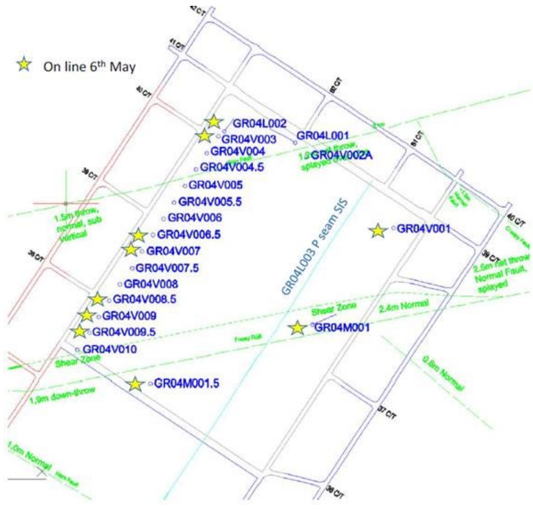
Figure 126: Goaf wells on LW 104 - the stars denote those wells that were active at the time of the serious accident on 6 May 2020
