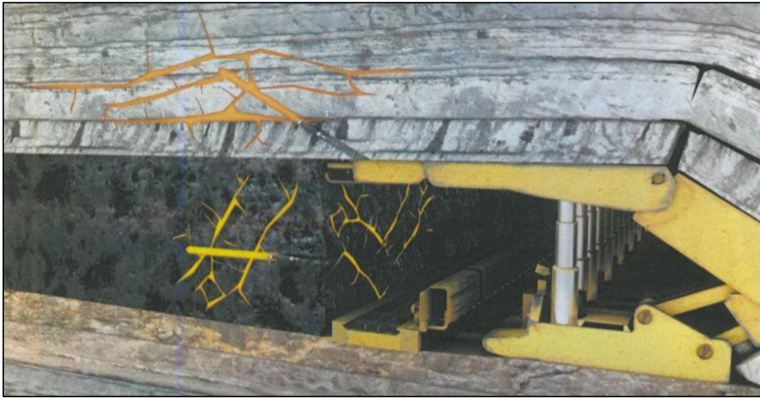
Figure 151: Example of the use of PUR for longwall face and roof consolidation
