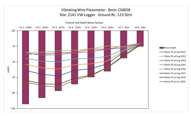
Figure E.2: Vibrating Wire Piezometer - Bore: CS4658 (Site 2141)
