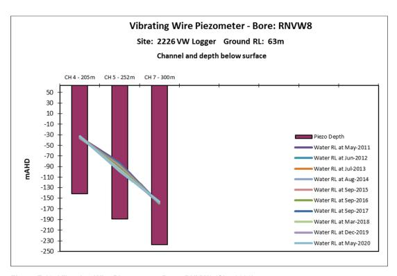
Figure E.10: Vibrating Wire Piezometer - Bore: RNVW8 (Site 2226)
