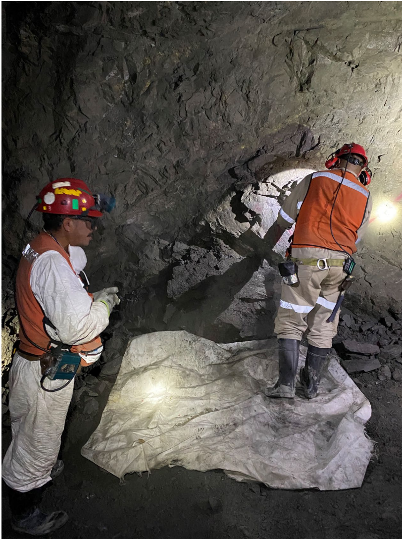
Figure 7-4: Rock Sampling: Use of Textile to Collect Rock Chips
