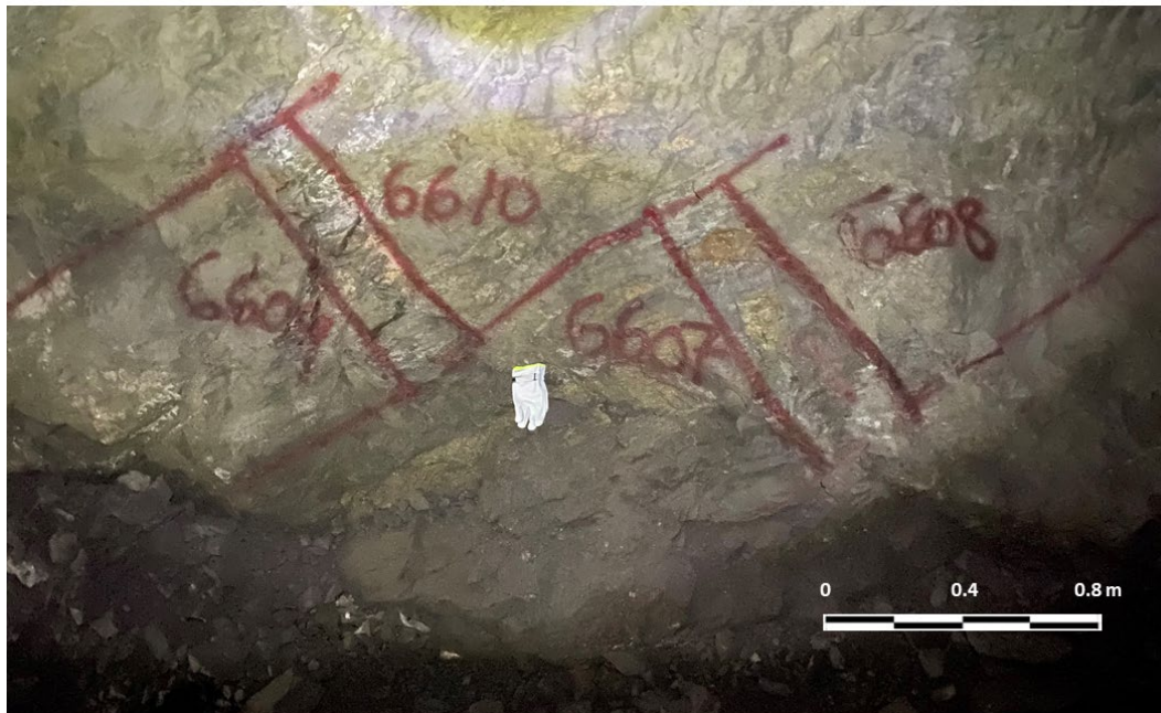
Figure 7-3: Marks Indicating Limits and Width of Samples
