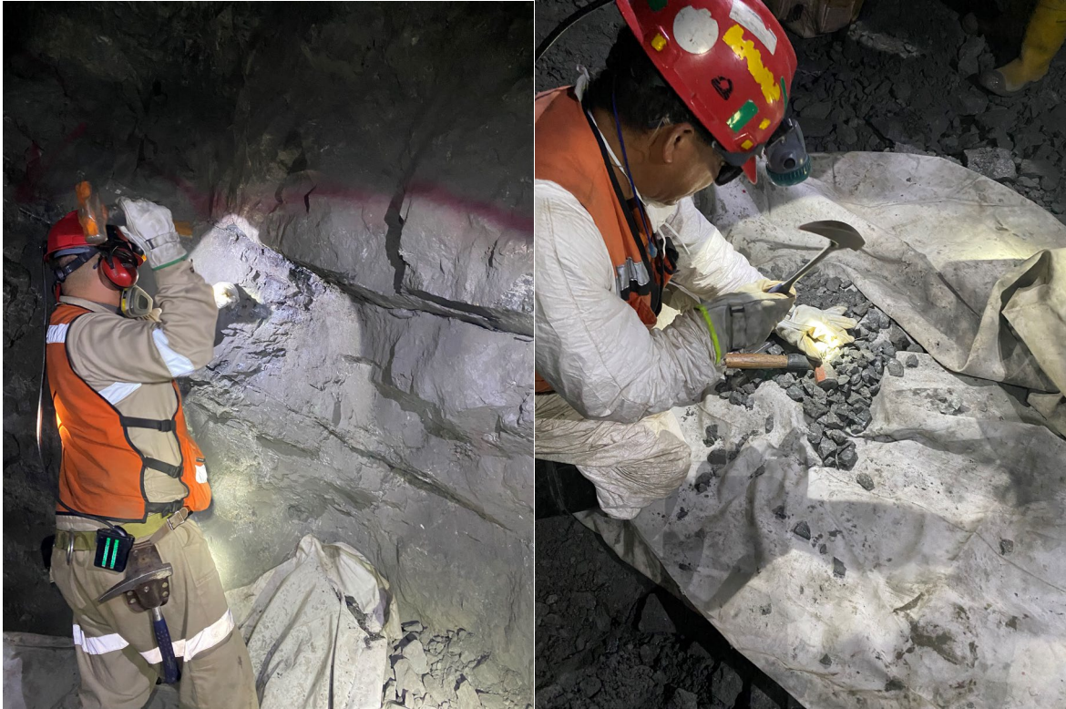
Figure 7-5: Left: Rock Sampling using Hammer and Chisel. Right: Homogenization of Fragments Size
