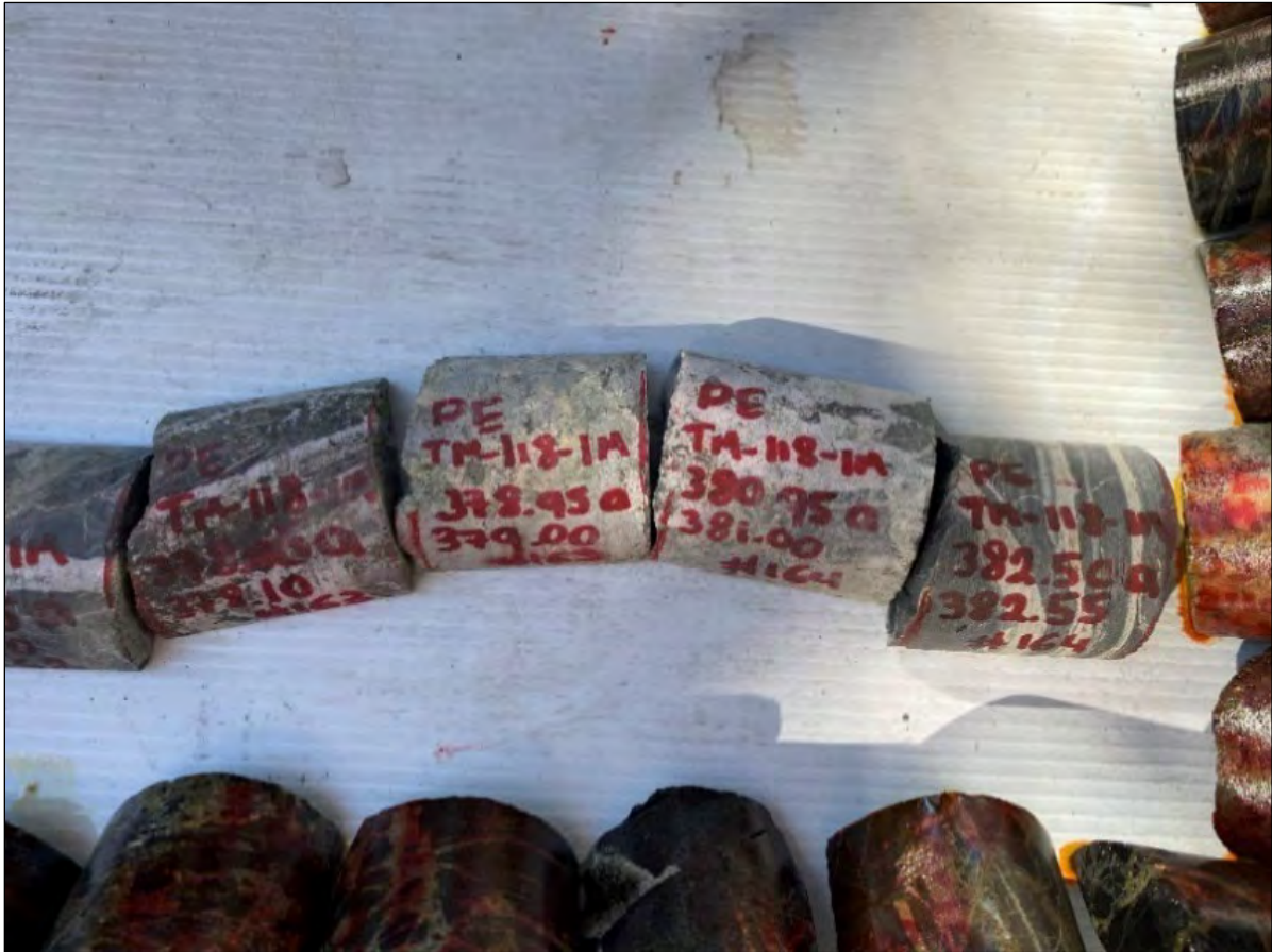
Figure 8.2: Core Samples Selected for Specific Gravity Testing
