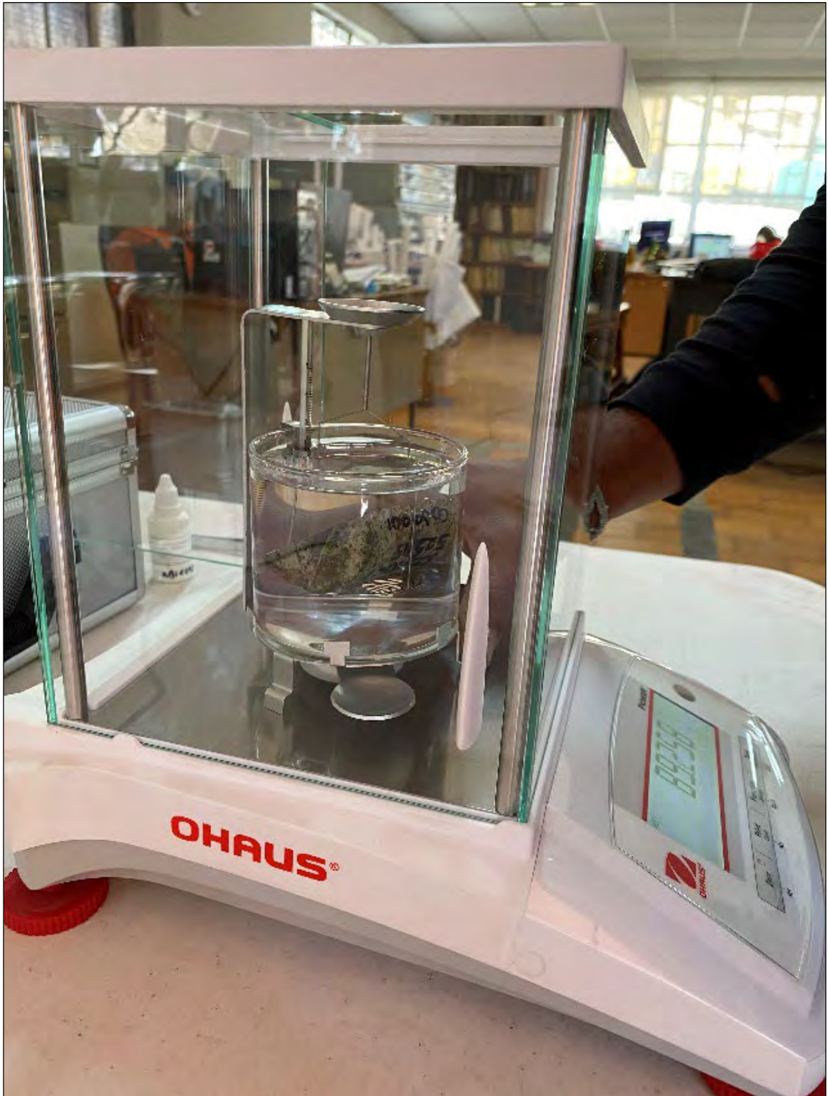
Figure 8.5: Weighting of the Sample Submerged in Water
