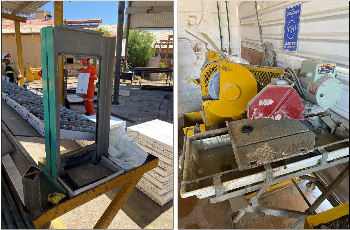
Figure 7.13: Core Splitter and Electrical Saw used at Santa Bárbara
