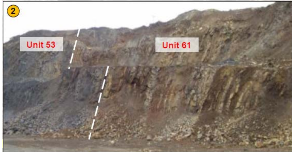
Figure 7.5: Contact Between Basal Silicates (Unit 61) and the Lower Member (53) in the Pit Wall
