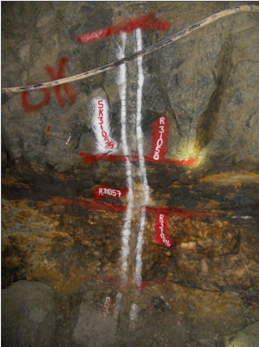
Figure 9-4: Channel Sampling Completed by GCM During 2016 Sampling Program
