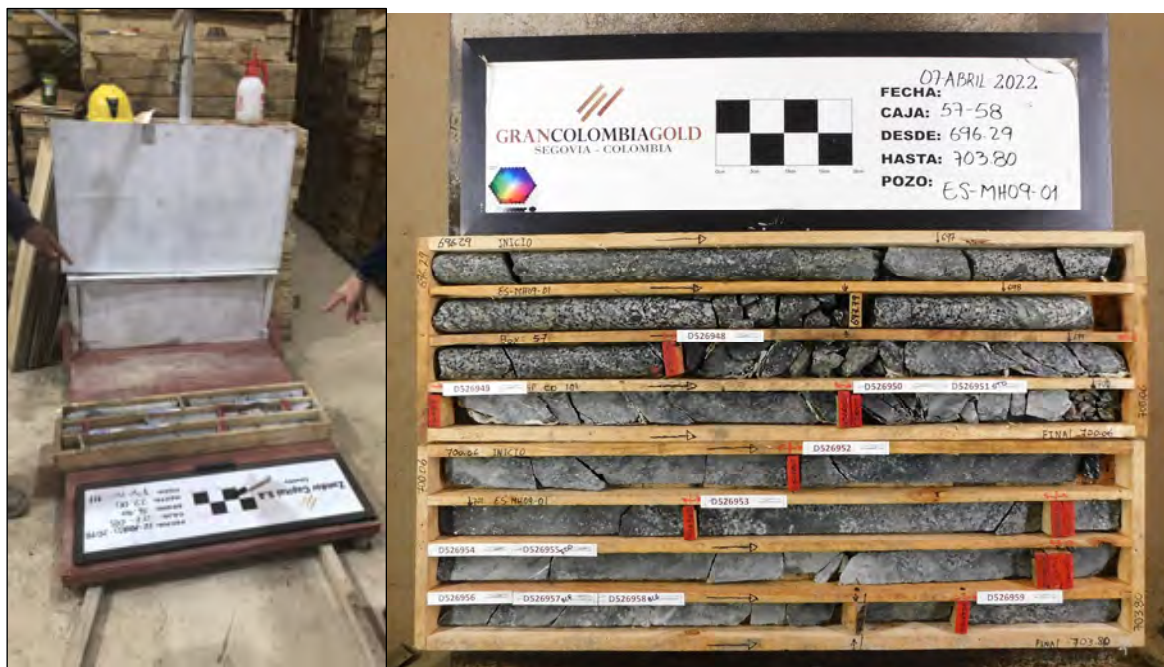
Figure 10-6: Example of Core Photography Setup (left) and Core Photographs (right)
