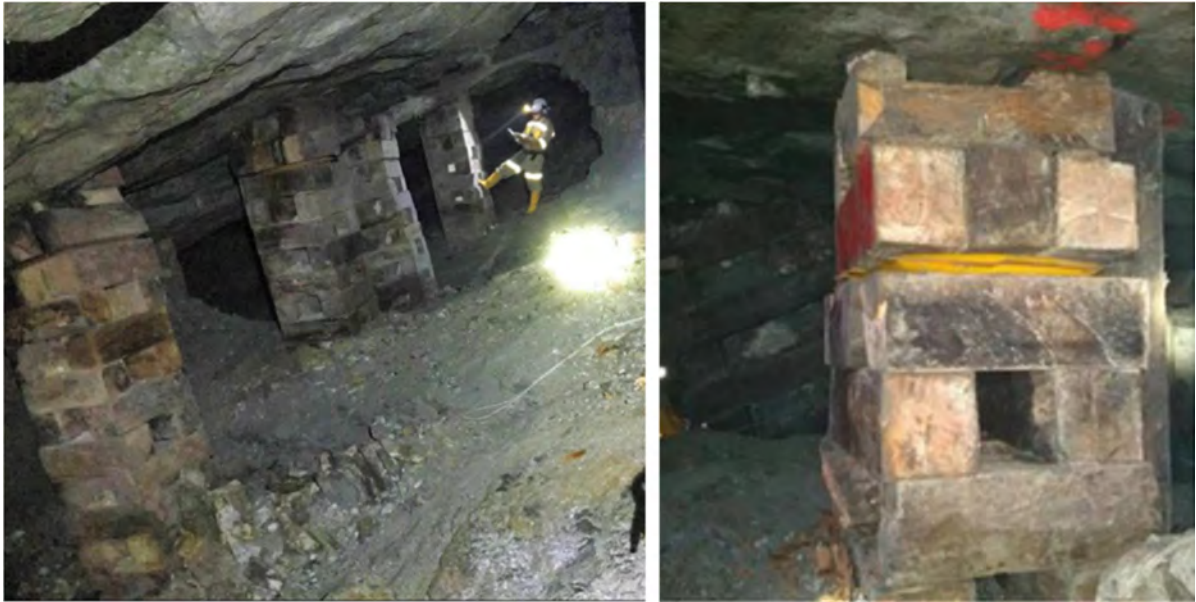
Figure 16-6: Timber Packs Example Used by Segovia
