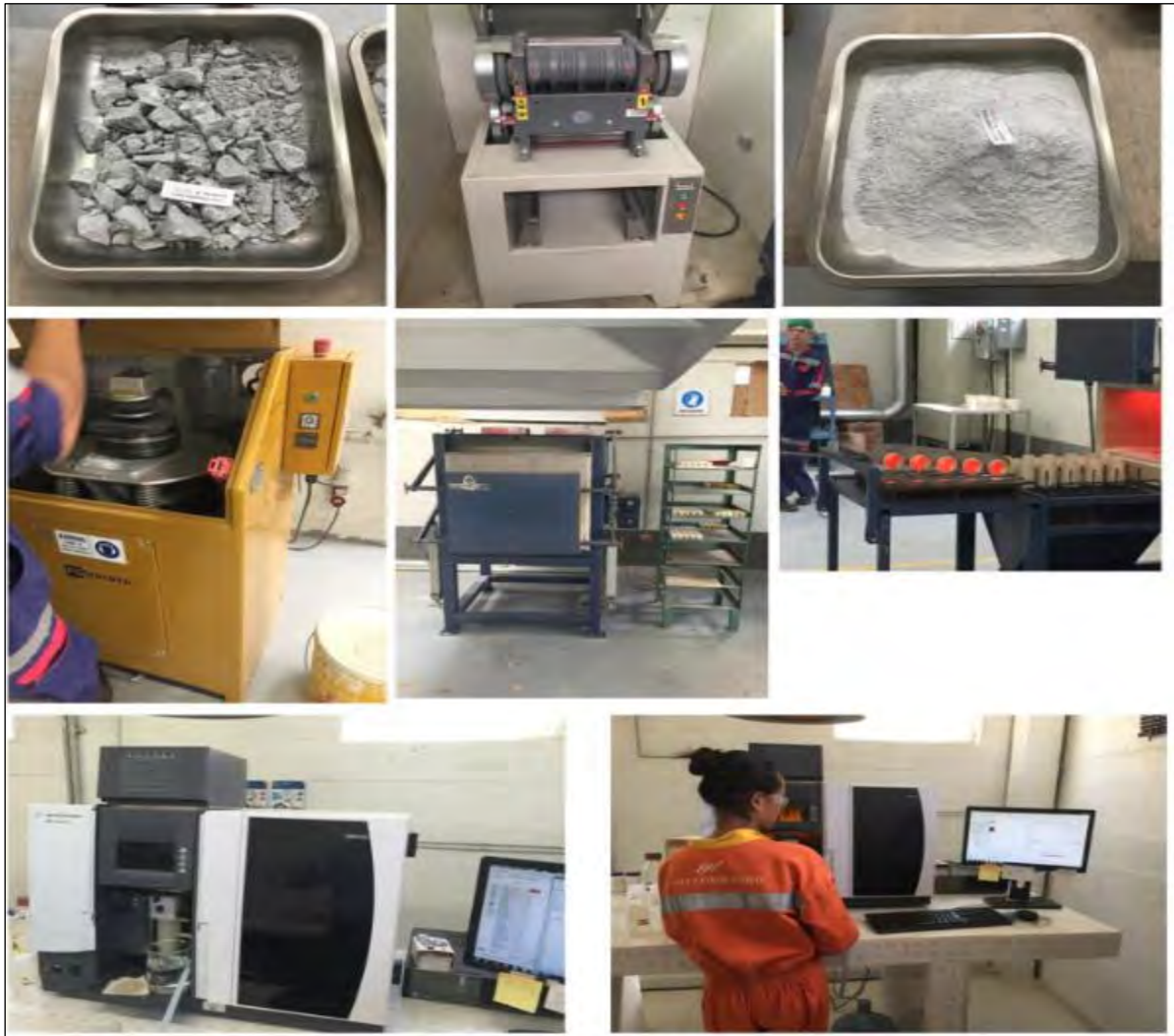
Figure 11-2: Mine Laboratory at Segovia, Showing Crusher, Pulverizer, Furnace and AA Assay Capture
