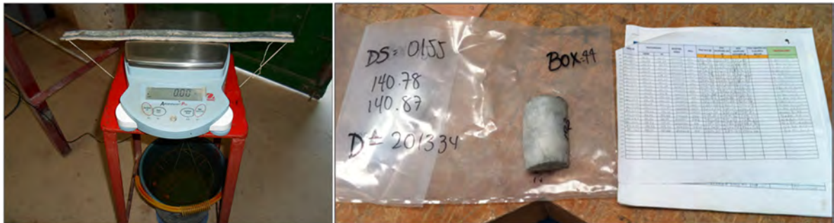
Figure 11-3: Core Sample Coated in Paraffin Wax with Logging Sheet, Prior to Entry to the Database
