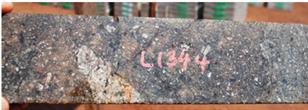
Figure 7.8: Phonolite Dyke in Drill Core, Lightly Fenitised with Phenocrysts of K-Feldspar and Nepheline and a Xenolith of Coarse-Grained Nepheline Syenite
