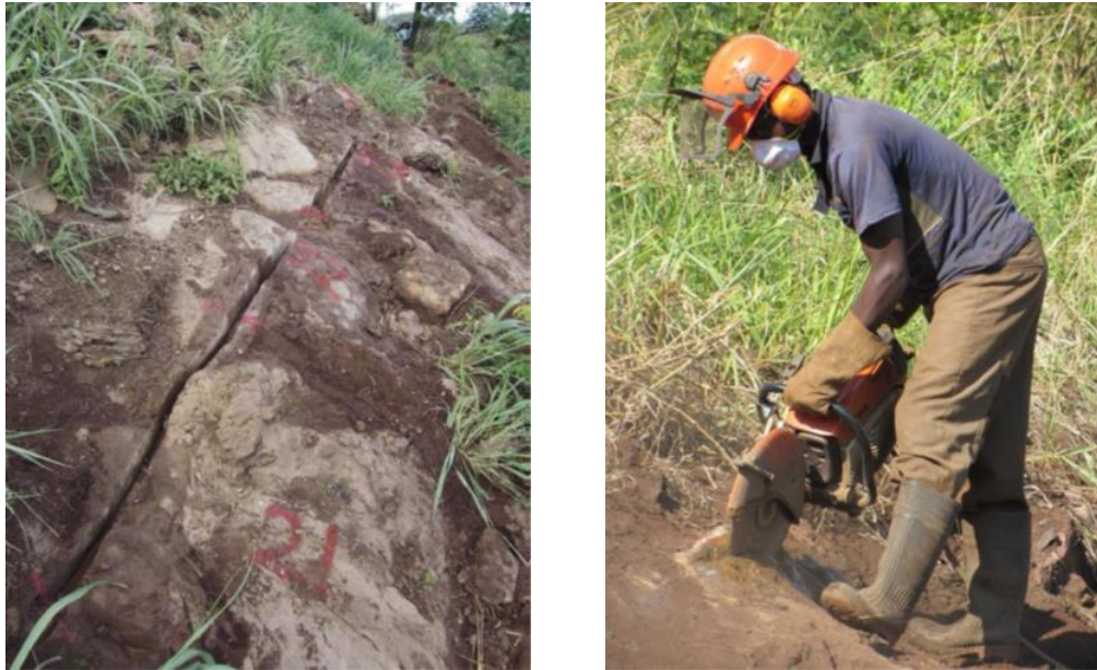
Figure 9.12: Example of Channel Sampling Programme on Songwe Hill
