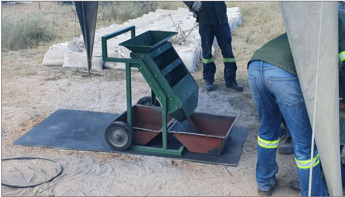
Figure 12-2: Riffle splitter used for the RC sample reduction process
