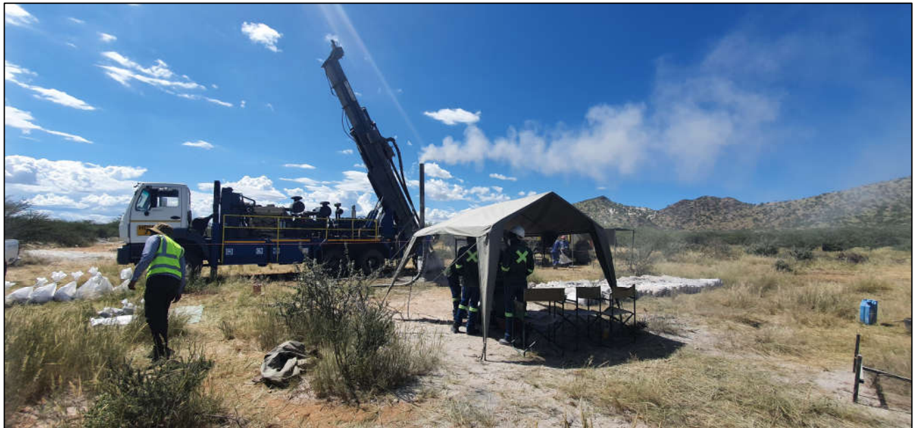
Figure 12-1: Operating RC rig drilling OKR296 with sample reduction area in foreground
