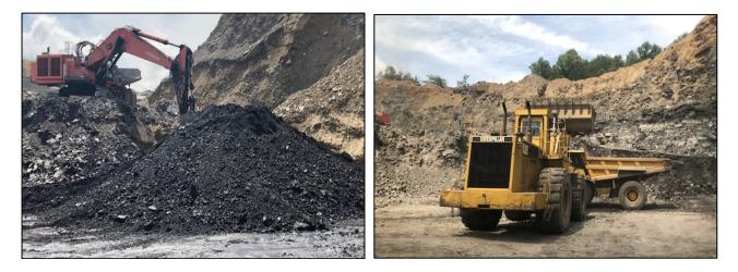
Frequently at the BWM Mine waste removal and coal recovery is double handled with excavators and front end loaders as opposed to loading direct into haul trucks.
