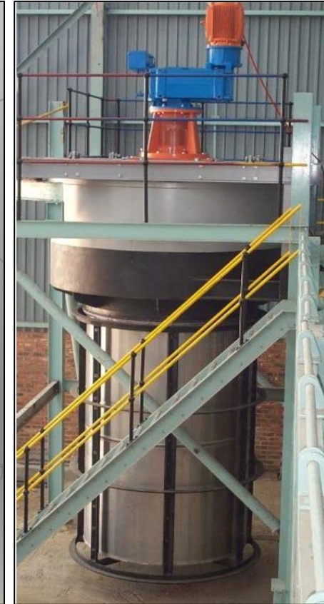
Assembled Kemix interchange screen (sample)
