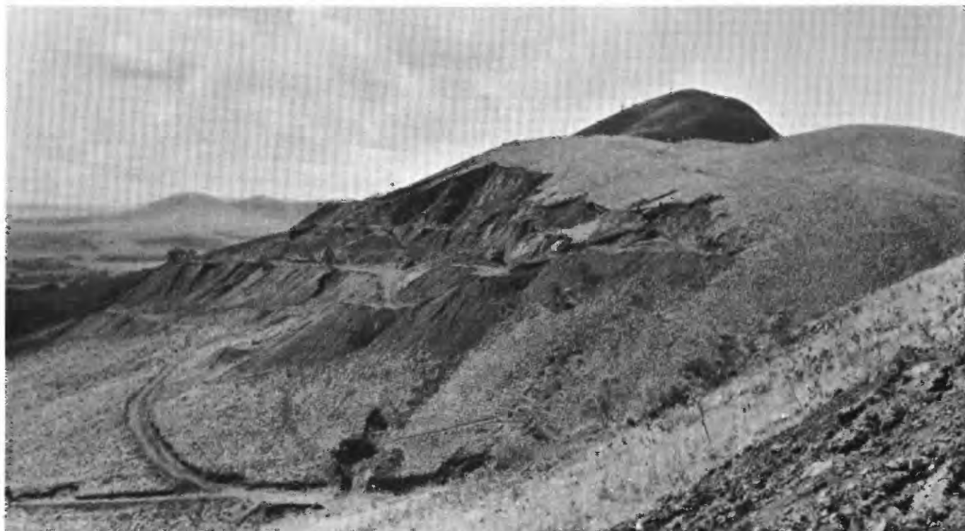
FIGURE 23.—Open-pit manganese mine in the Serra da Moeda near Lagoa Grande. The manganese ore forms lenses in the contact zone between the Cauê Itabirite (top of ridge) and the Gandarela Formation (flank of ridge).
