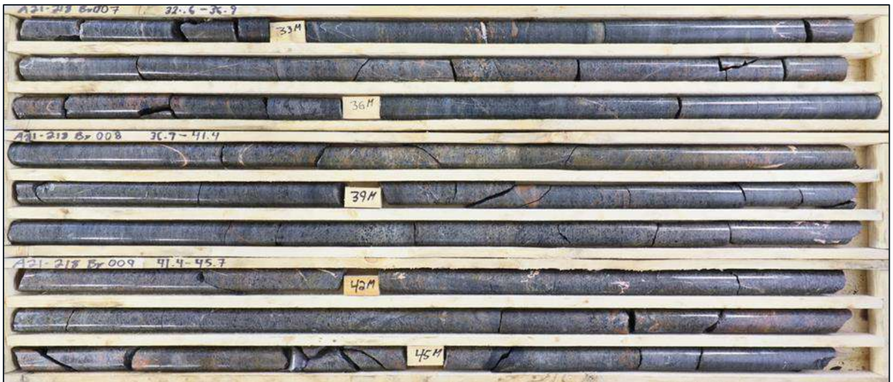
Figure 7-13: Photograph of a Hangingwall Gabbro Intersection from A21-213 Between 32.6 and 45.7 m (NQ Core Diameter, Box Length 1.5 m).
