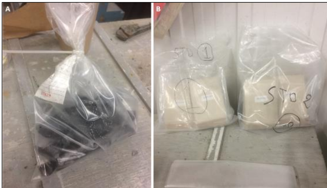
Figure 11-2 A) Sample in Plastic Bag with Tag; B) Two Standards used during the Drilling Program
