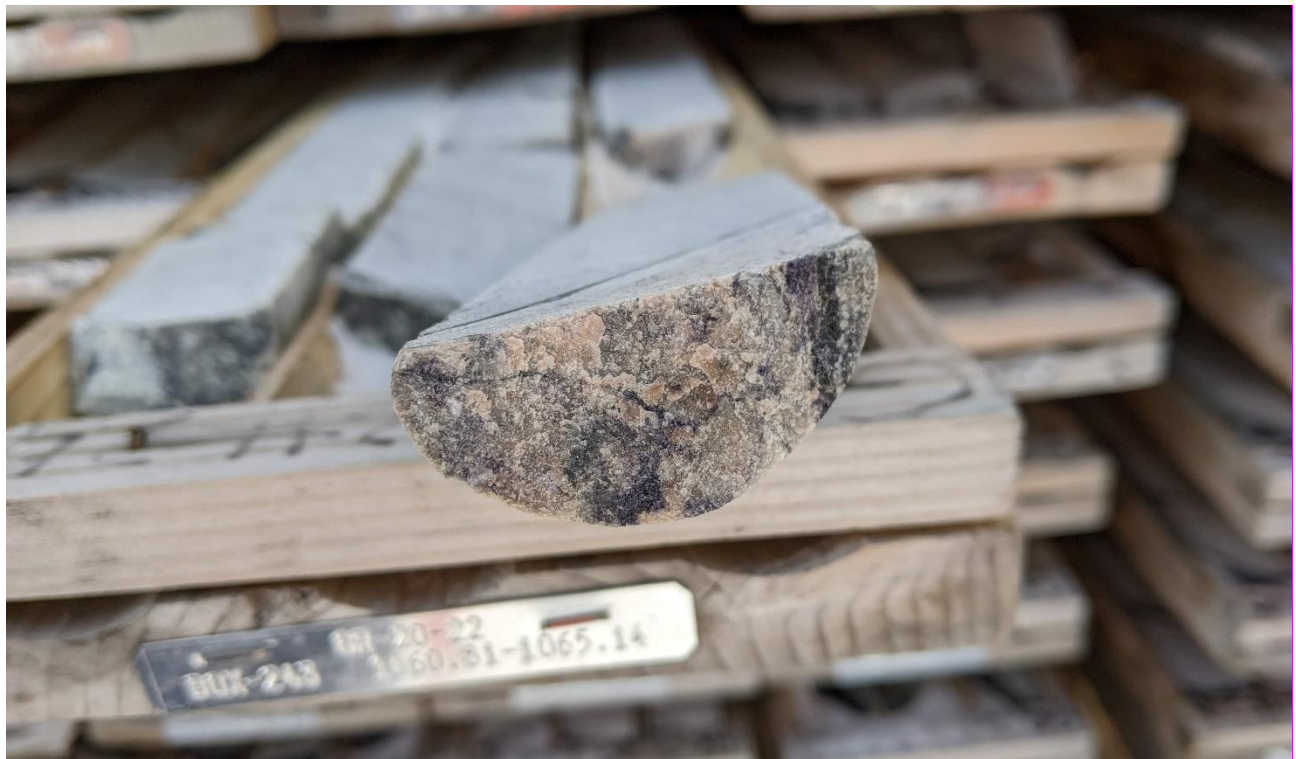
Figure 12-11 GR-20-22 from 1060 to 1065 m with Purple Mineral as Fracture Filling
