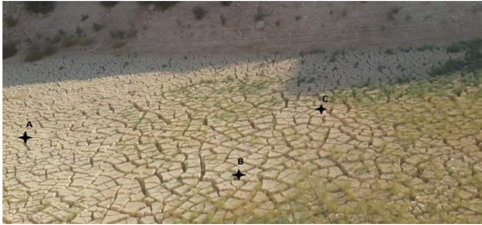
Figure 1: Abandoned mine filled with phosphate wash water after solar drying (marks A, B and C are the positions of samples)
