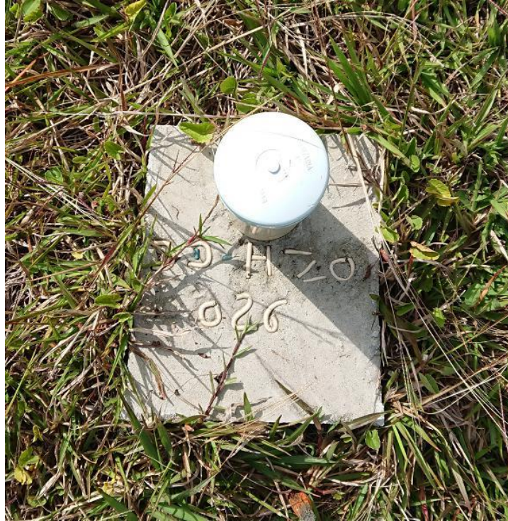
Figure 10-2: Collar Monument of DDH-ZO-026 at La Cumbre Area
