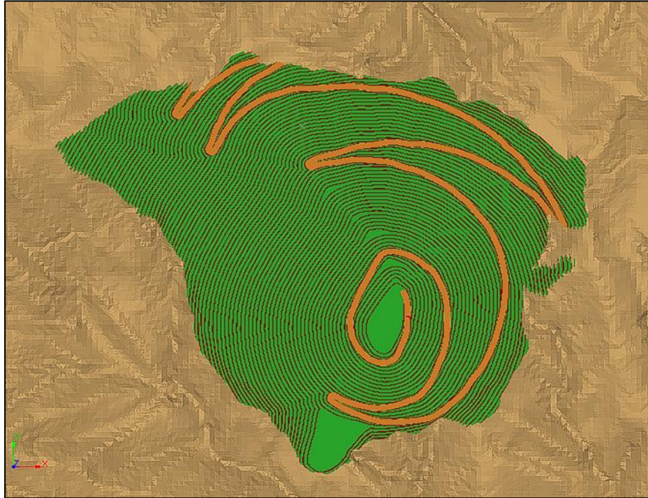
Figure 16-13: La Cumbre Final Pit with Ramp Access
