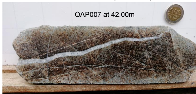
Figure 10-6: Drillhole QAP007, Quartz “B” Type Veinlet Hosted in a Porphyry Diorite with Strong Potassic Alteration (fine biotite)
