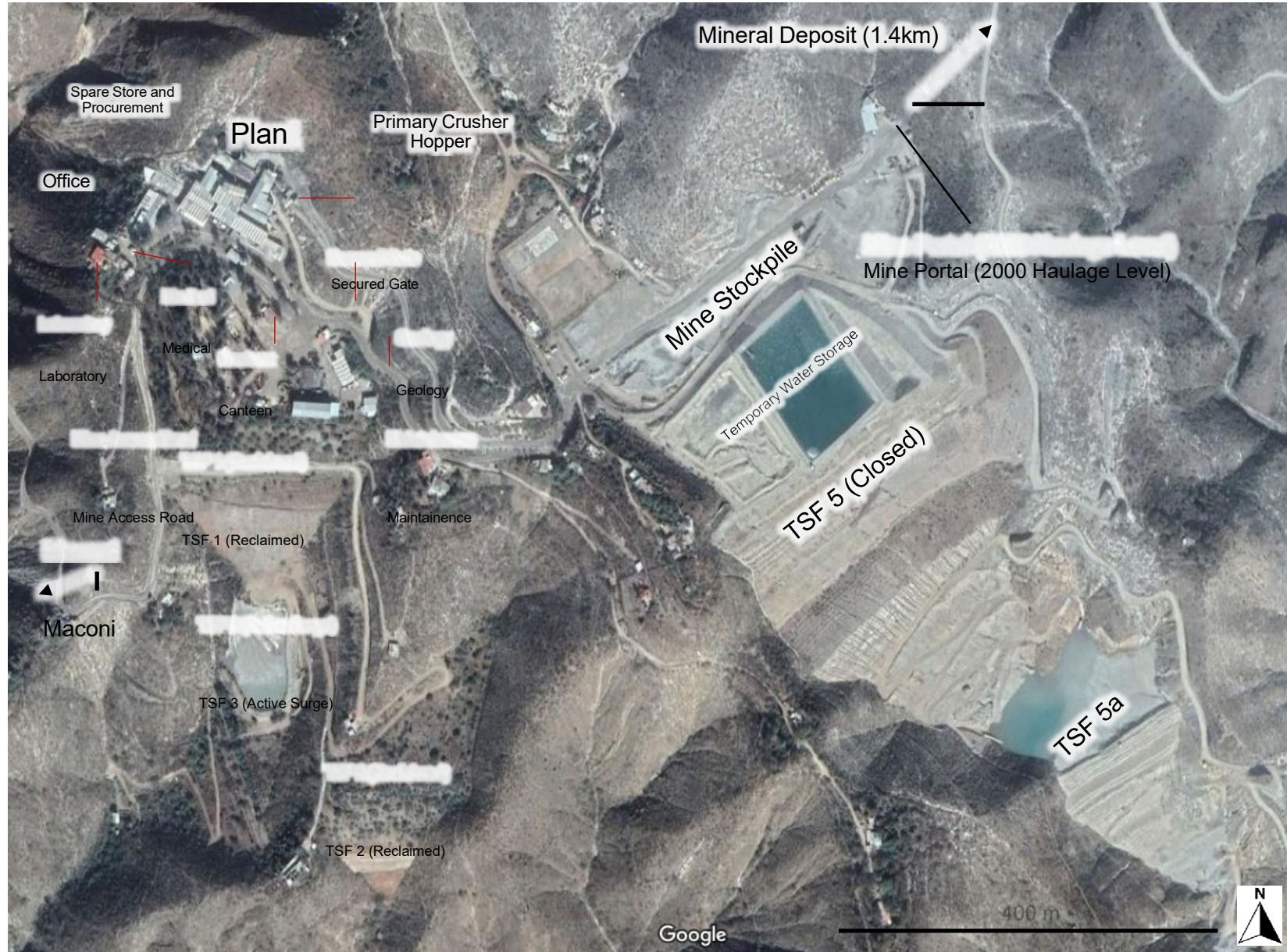
Figure 5.2 Minera La Negra Layout and Infrastructure
