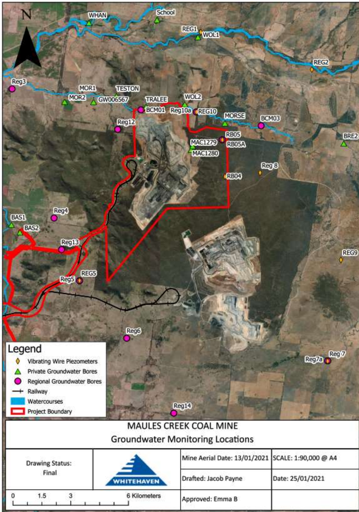
Figure 11 Groundwater Monitoring Locations
